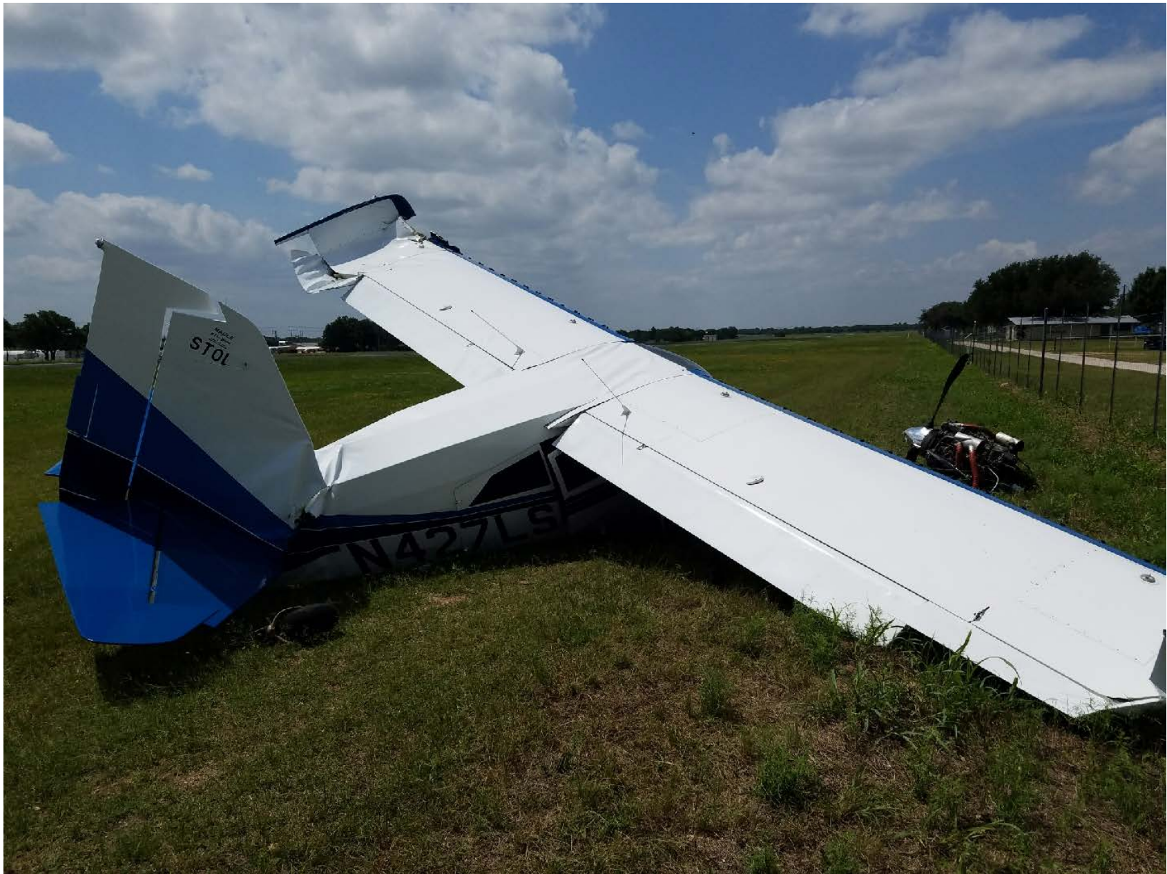
Photo 1 – View of damage to left wing and aft fuselage (Courtesy of FAA)
