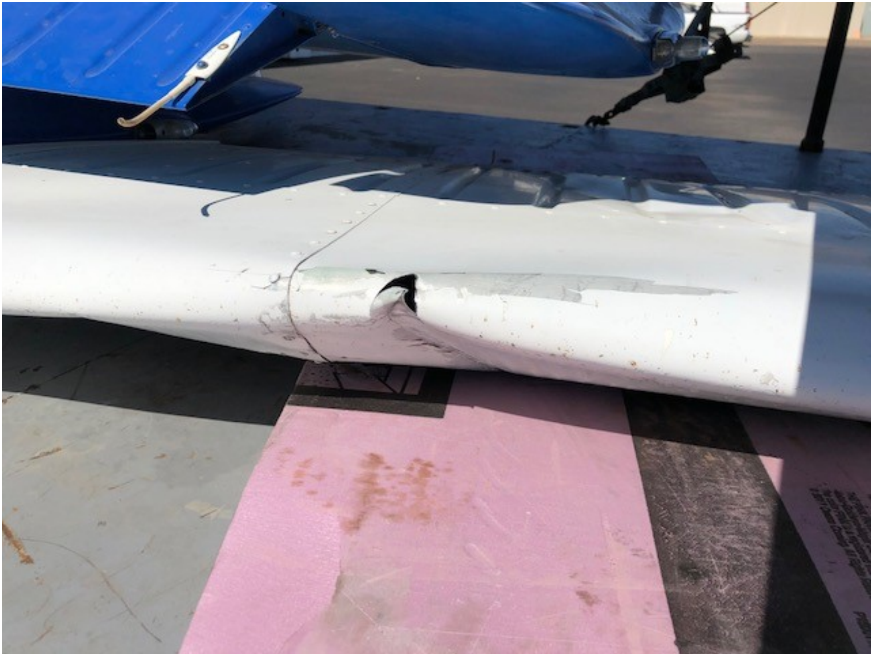
Photo 1 – View of damaged horizontal stabilator (Photo courtesy of the FAA)
