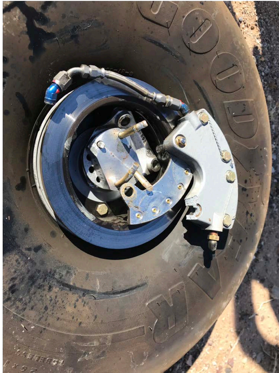
Photo 1 – View of separated right landing gear wheel and tire (Courtesy of FAA)
