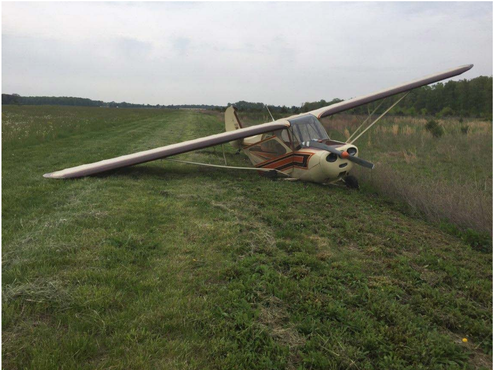
Photo 1 – View of damage to right wing lift struts (Courtesy of FAA)
