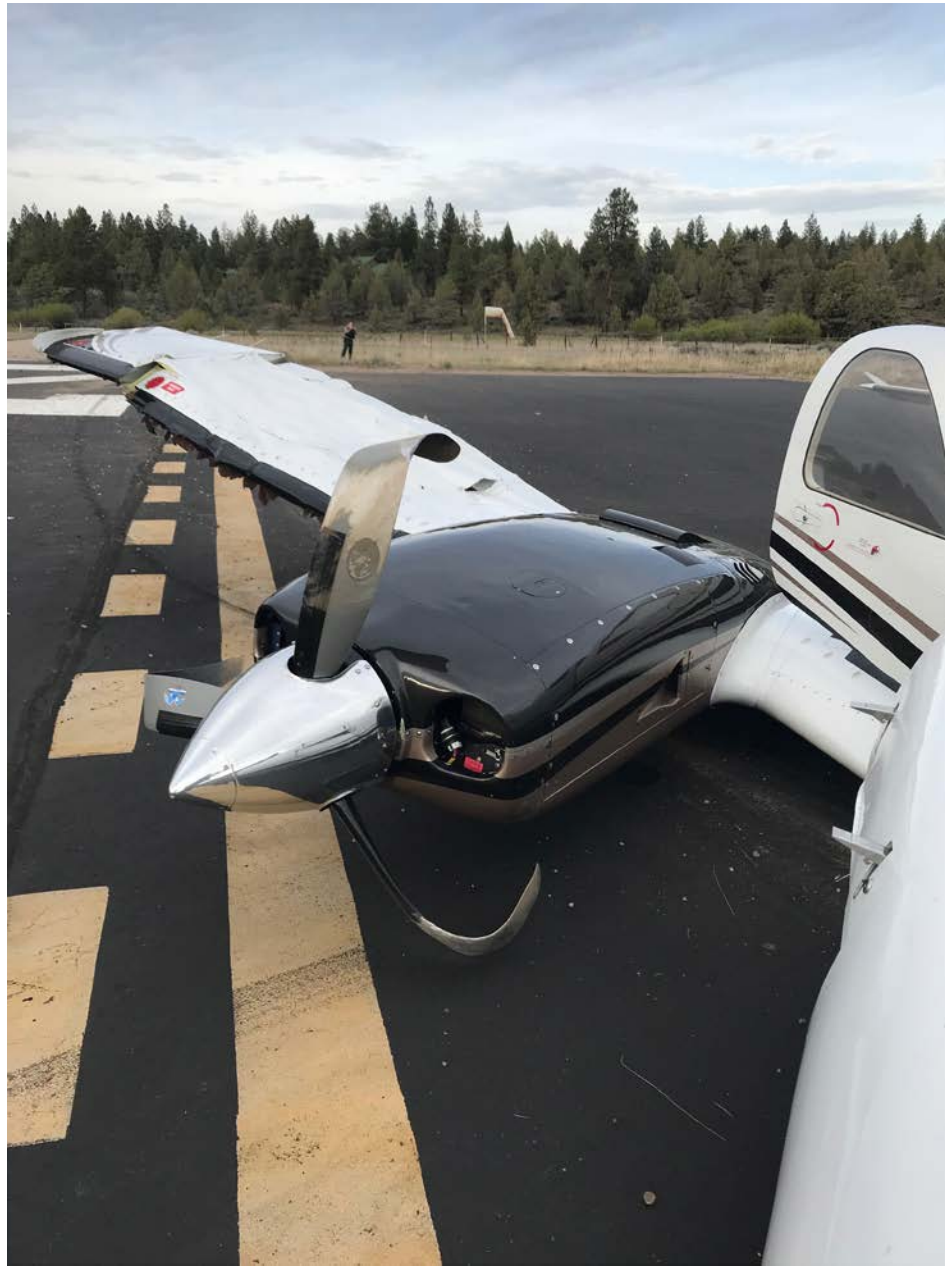
Photo 1 – View of damage to right wing spar (Courtesy of FAA)
