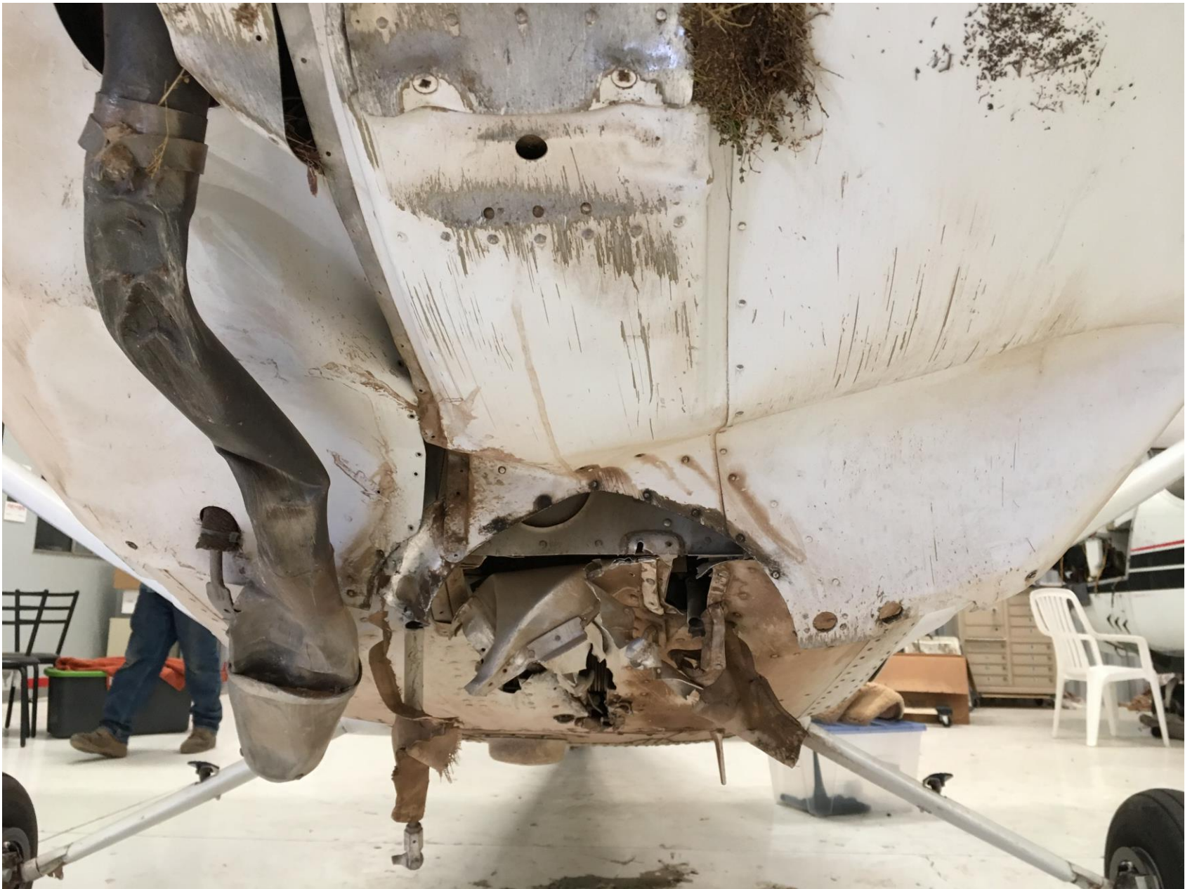
Photo 1 – View of damaged lower front fuselage (Photo courtesy of the FAA)
