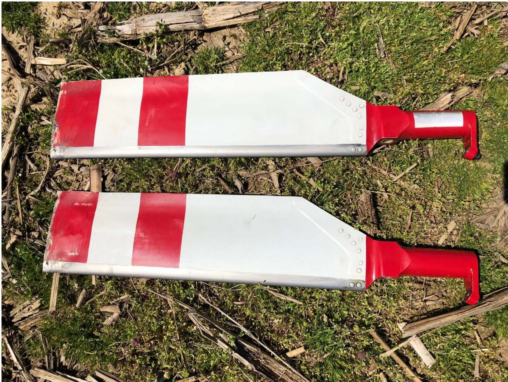
Photo 1 – View of damaged tail rotors (Photo courtesy of the Chief Pilot)
