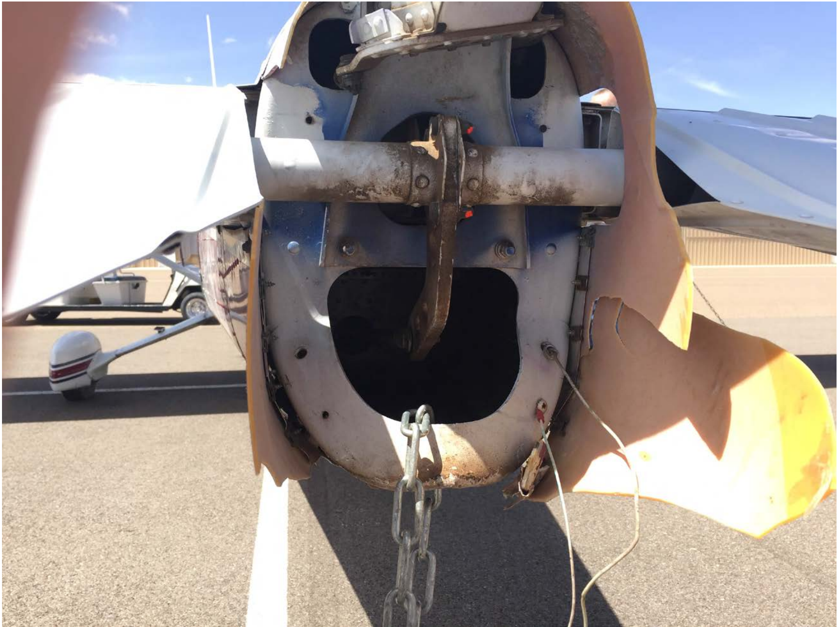
Photo 1 – View of damaged empennage (Photo courtesy unknown)
