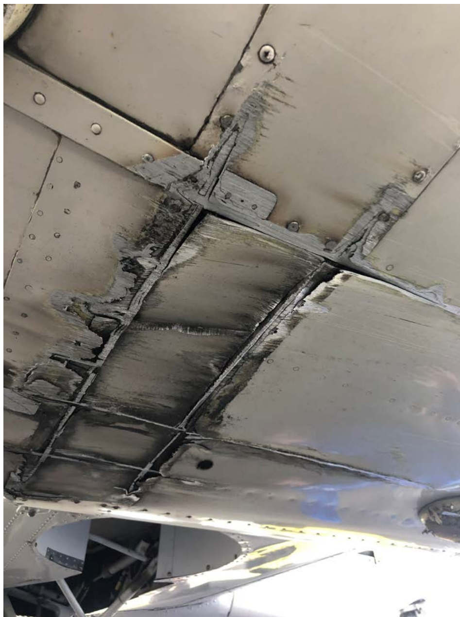
Photo 1 – View of damage to the longerons and spar carry through (Courtesy of FAA)
