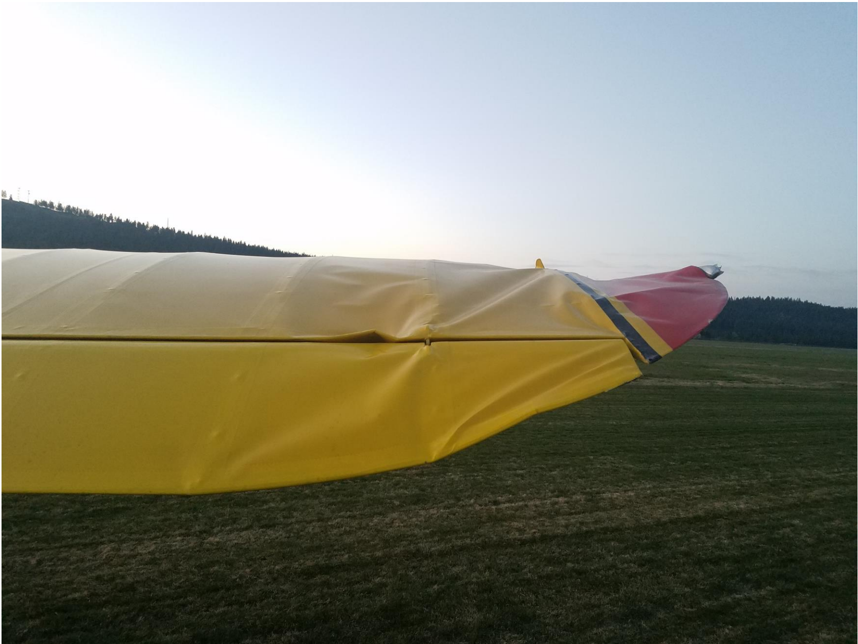
Photo 1 – Rear view of damaged right wing and aileron (Photo courtesy of the FAA)
