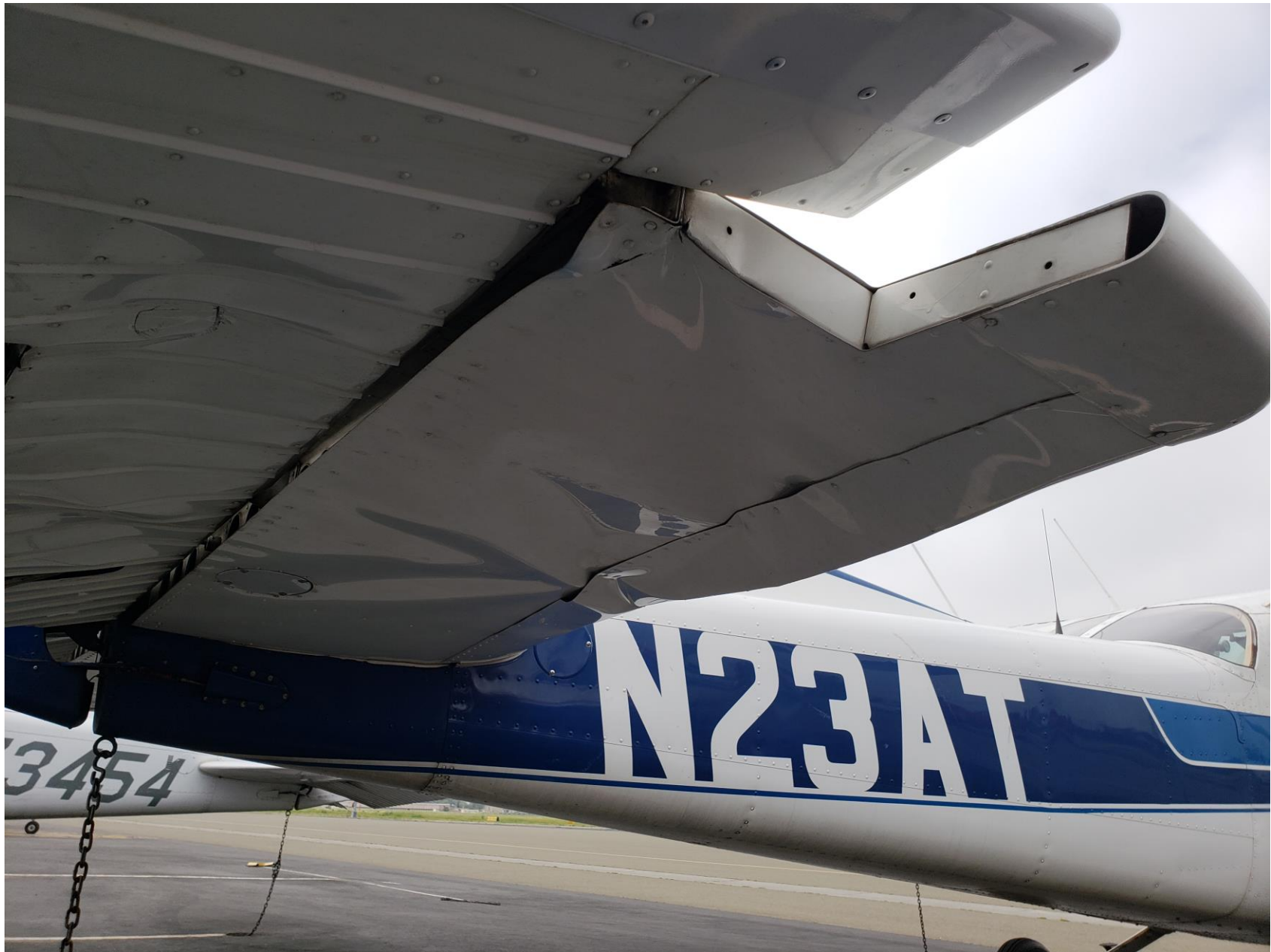
Photo 1 – View of bottom damaged horizontal stabilizer and elevator (Photo courtesy of the FAA)
