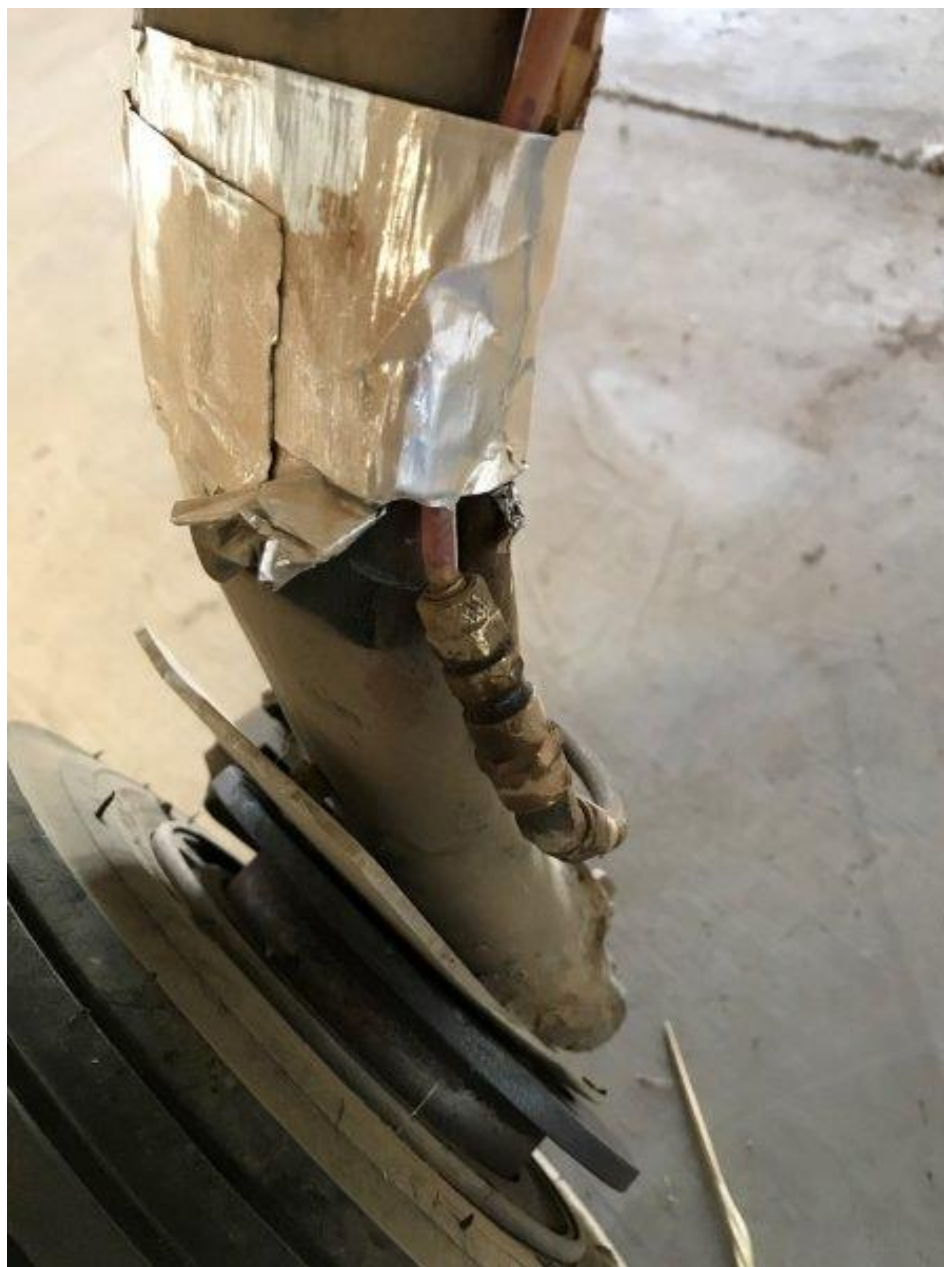
Photo 2 – View of damage to the right brake assembly (Courtesy of FAA)
