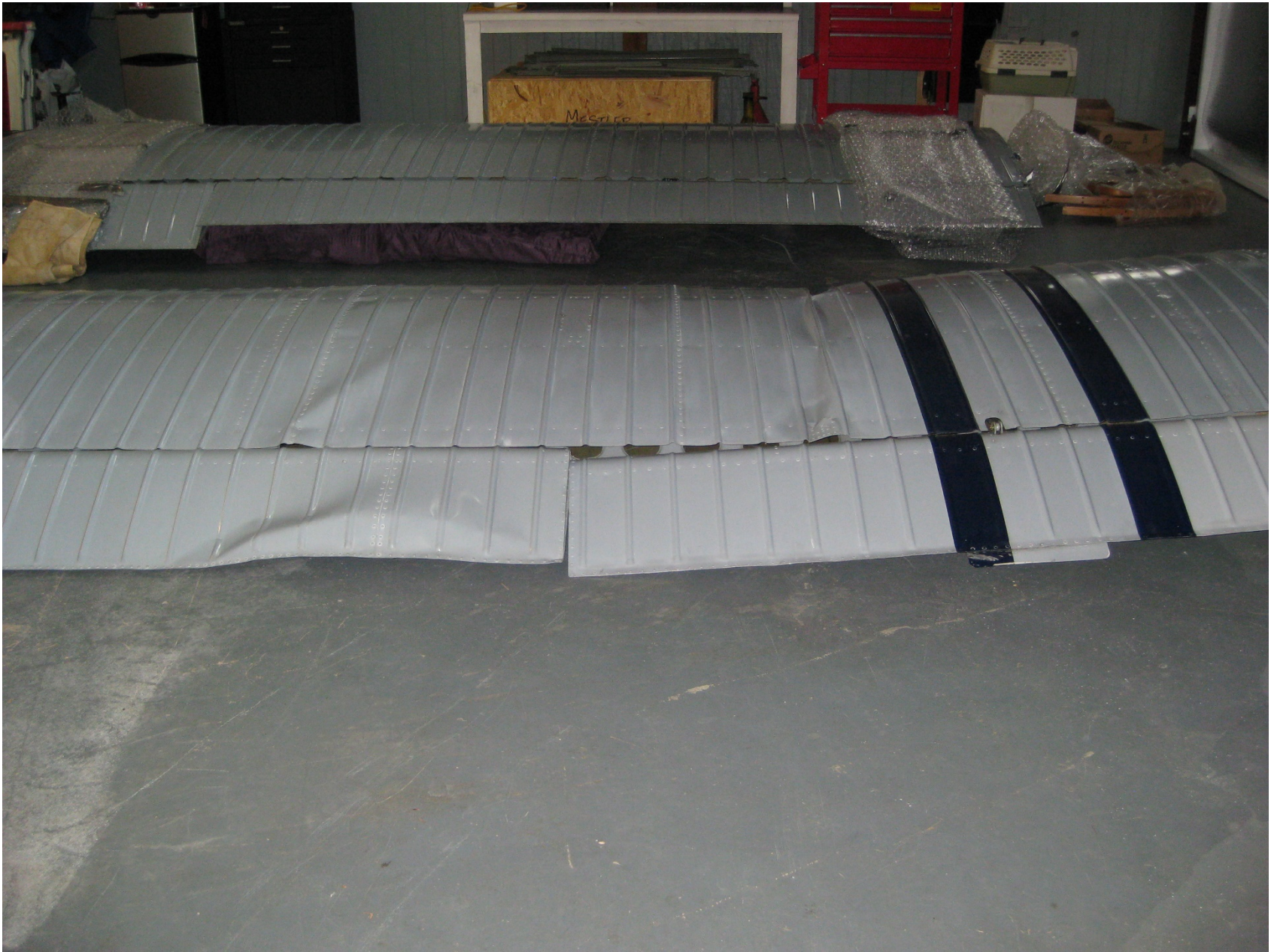
Photo 1 – View of right wing damage (Photo courtesy unknown)
