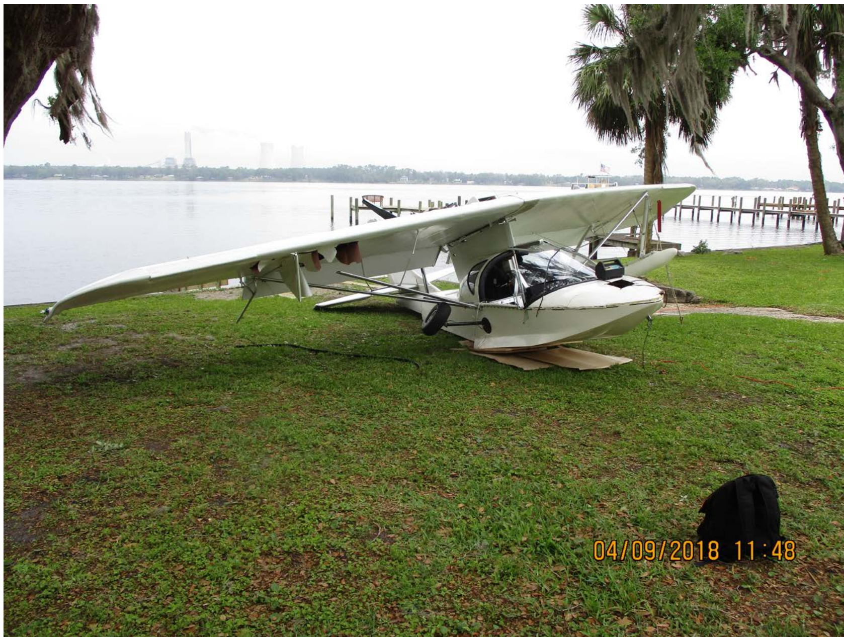
Photo 1 – View of damage to right-wing lift strut and windshield (Courtesy of FAA)
