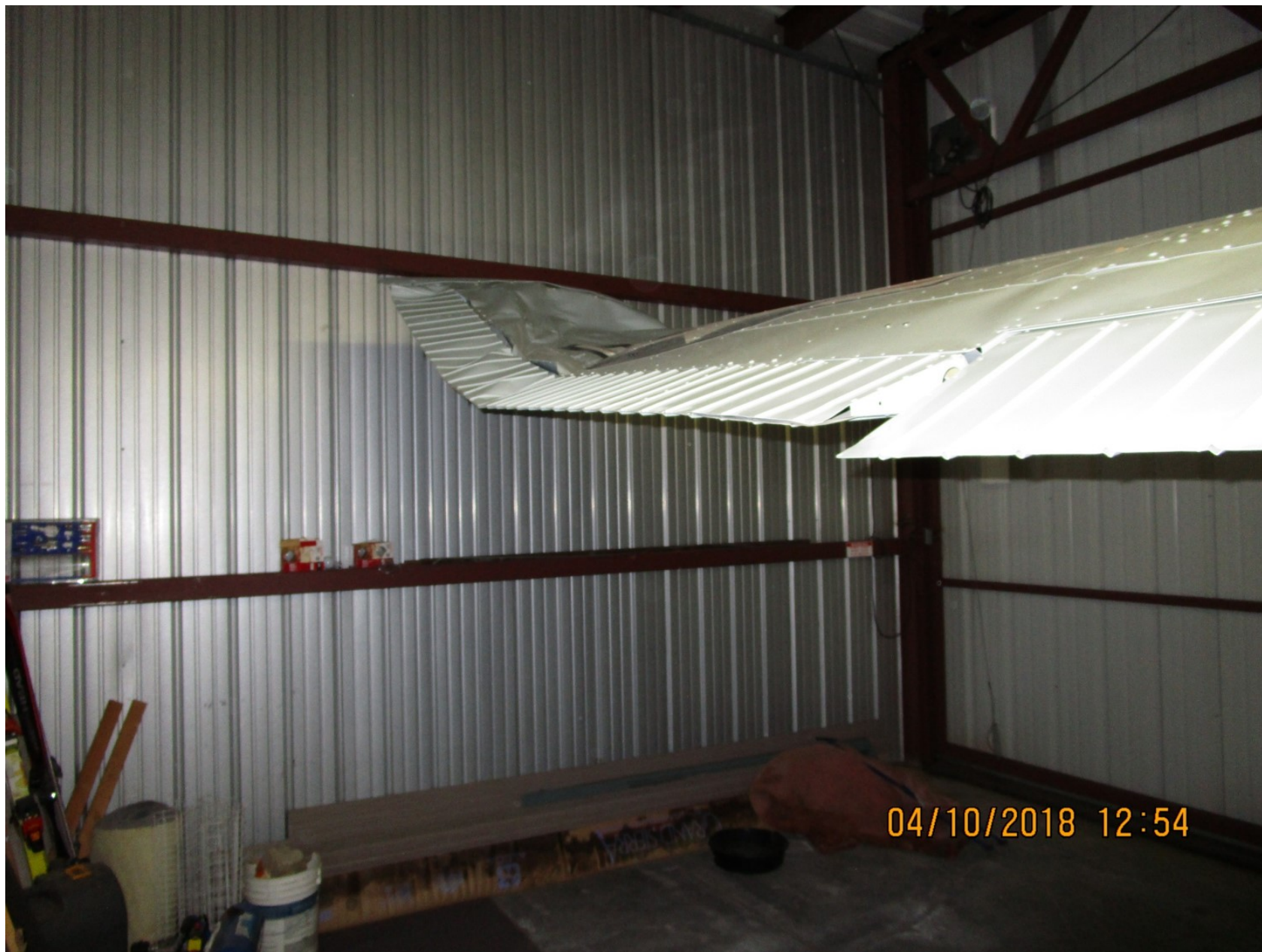
Photo 1 – View of damage to left wing spar and aileron (Courtesy of FAA)
