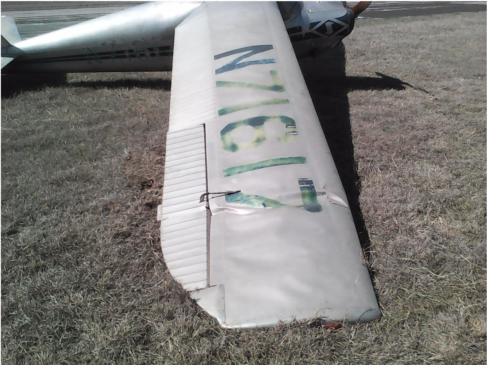
Photo 2 – View of damaged right wing and aileron (Photo courtesy of the FAA)
