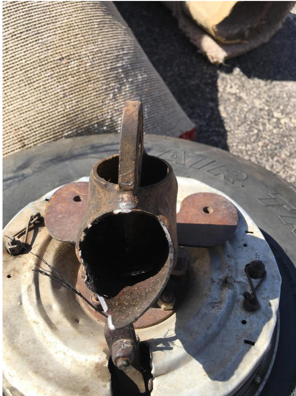
Photo 3 – View of separated right landing gear (Photo courtesy of the FAA)
