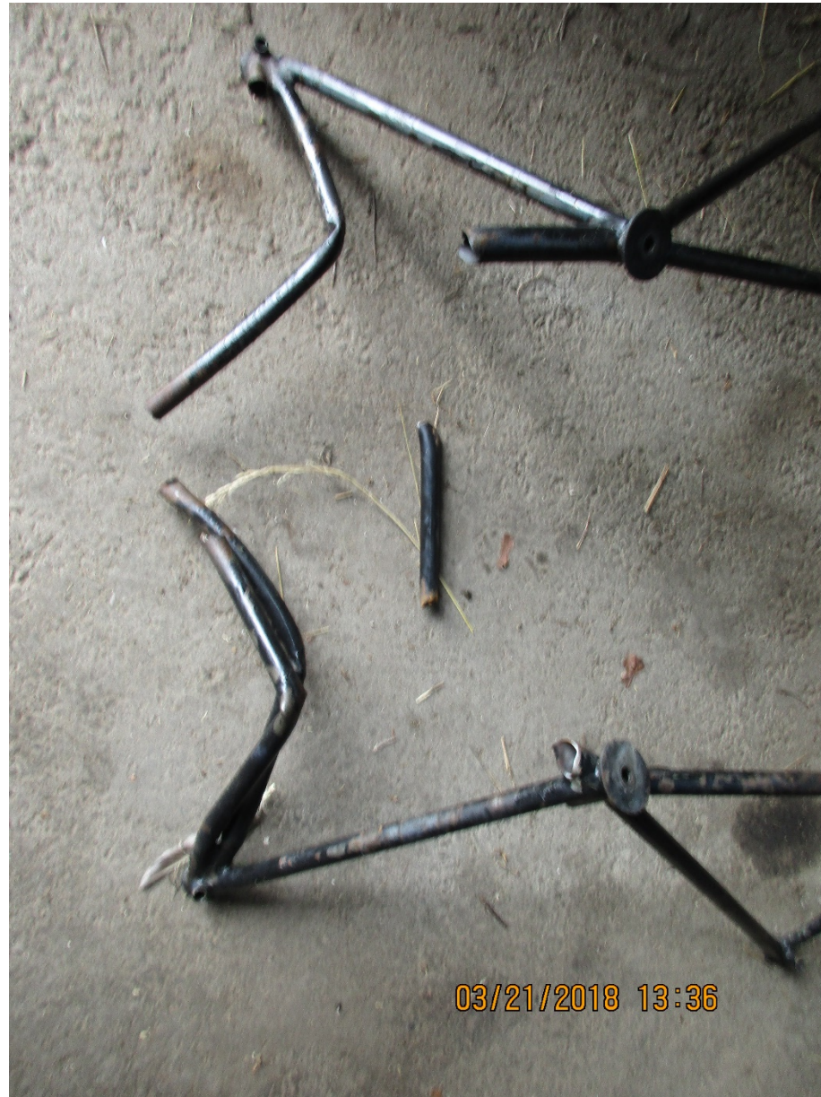
Photo 1 – View of damaged engine mounts (Photo courtesy of the FAA)
