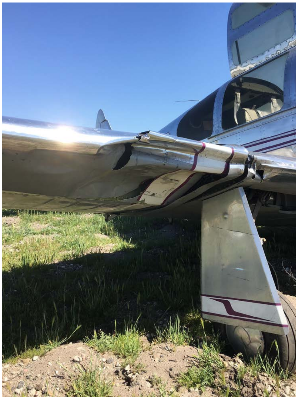
Photo 1 – View of damage to right wing (Courtesy of FAA)
