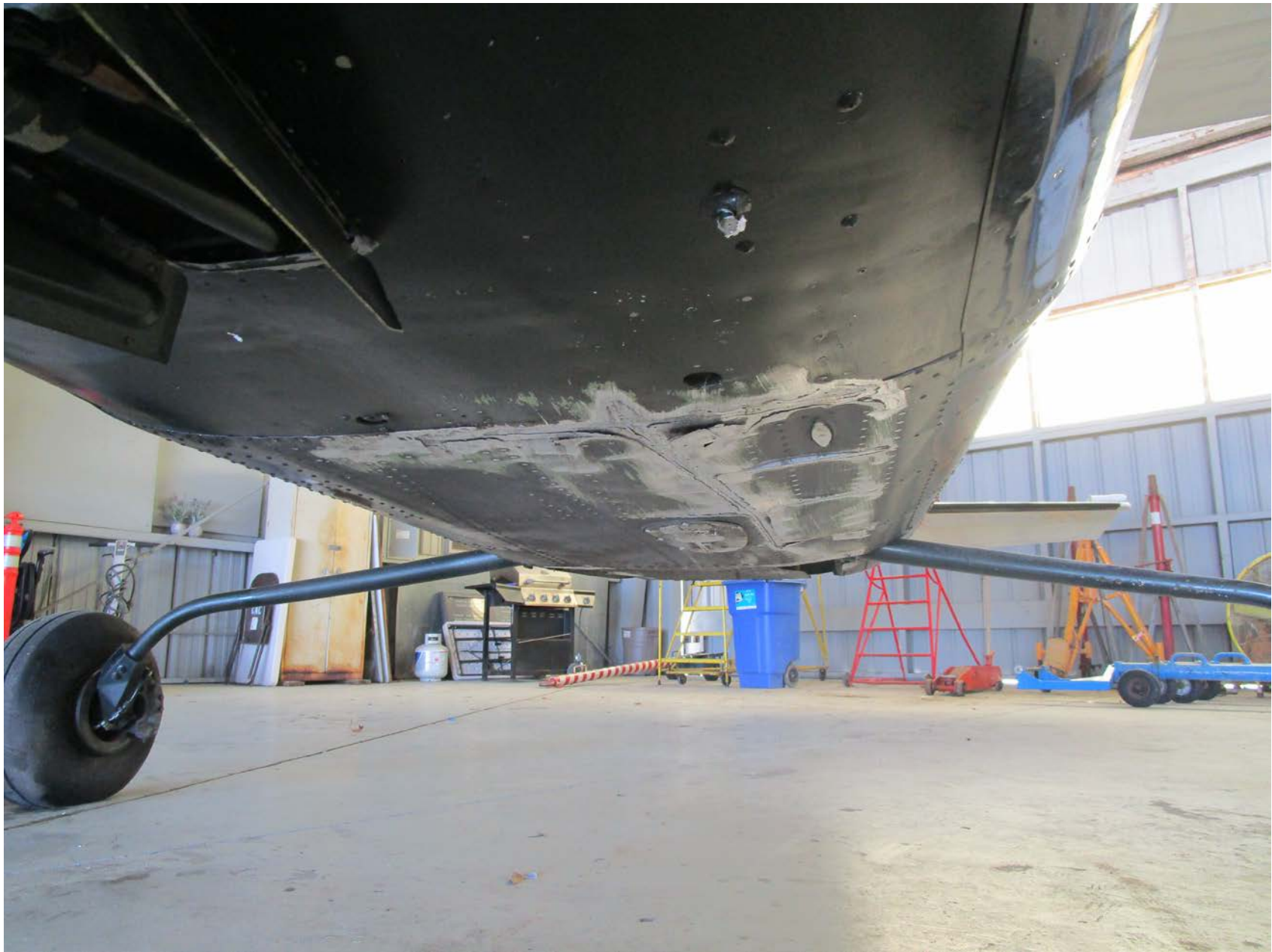
Photo 1 – View of damage to the lower fuselage longerons and bulkhead (Courtesy of FAA)
