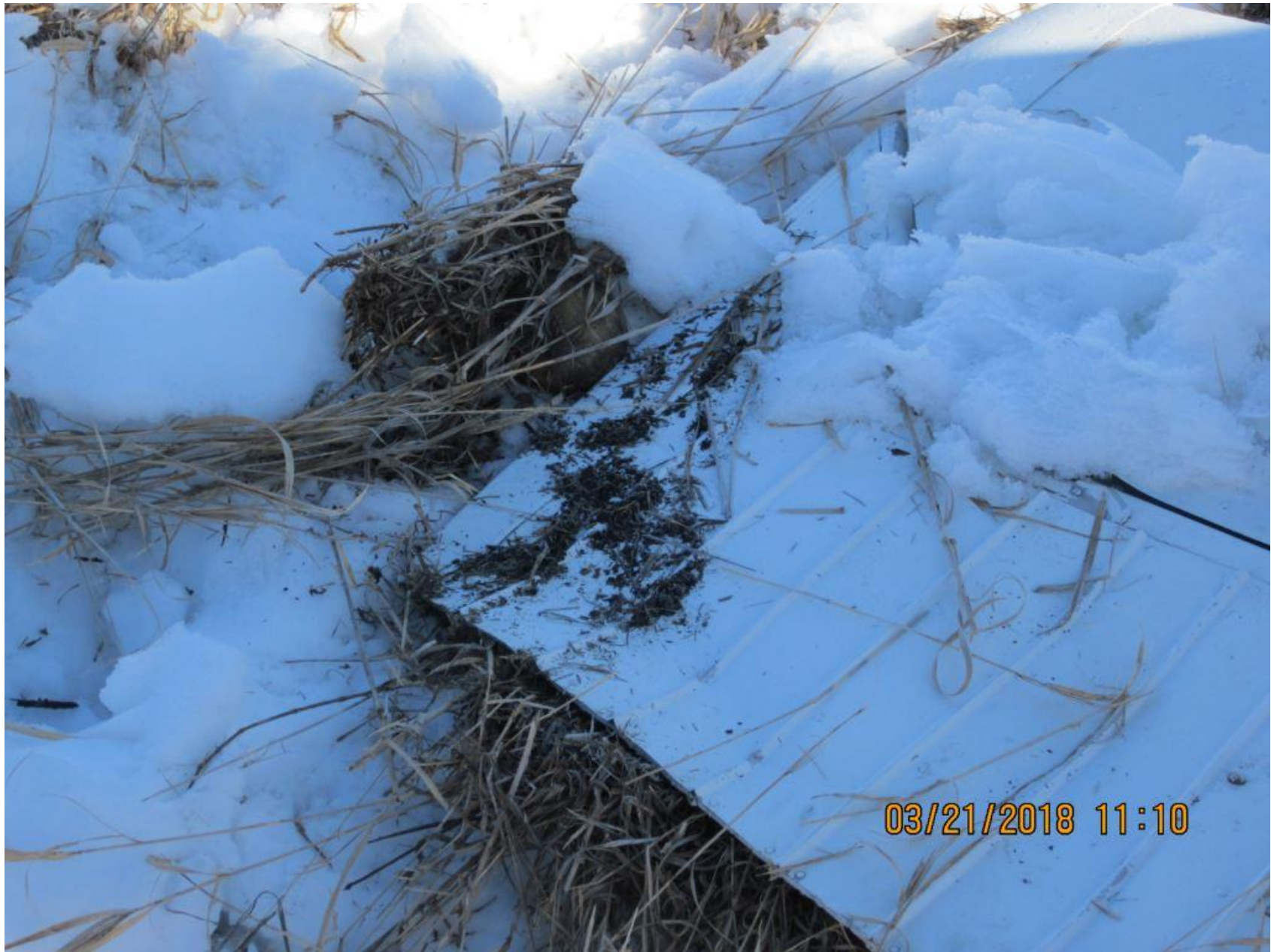
Photo 3 – View of damaged elevator (Photo courtesy of the FAA)
