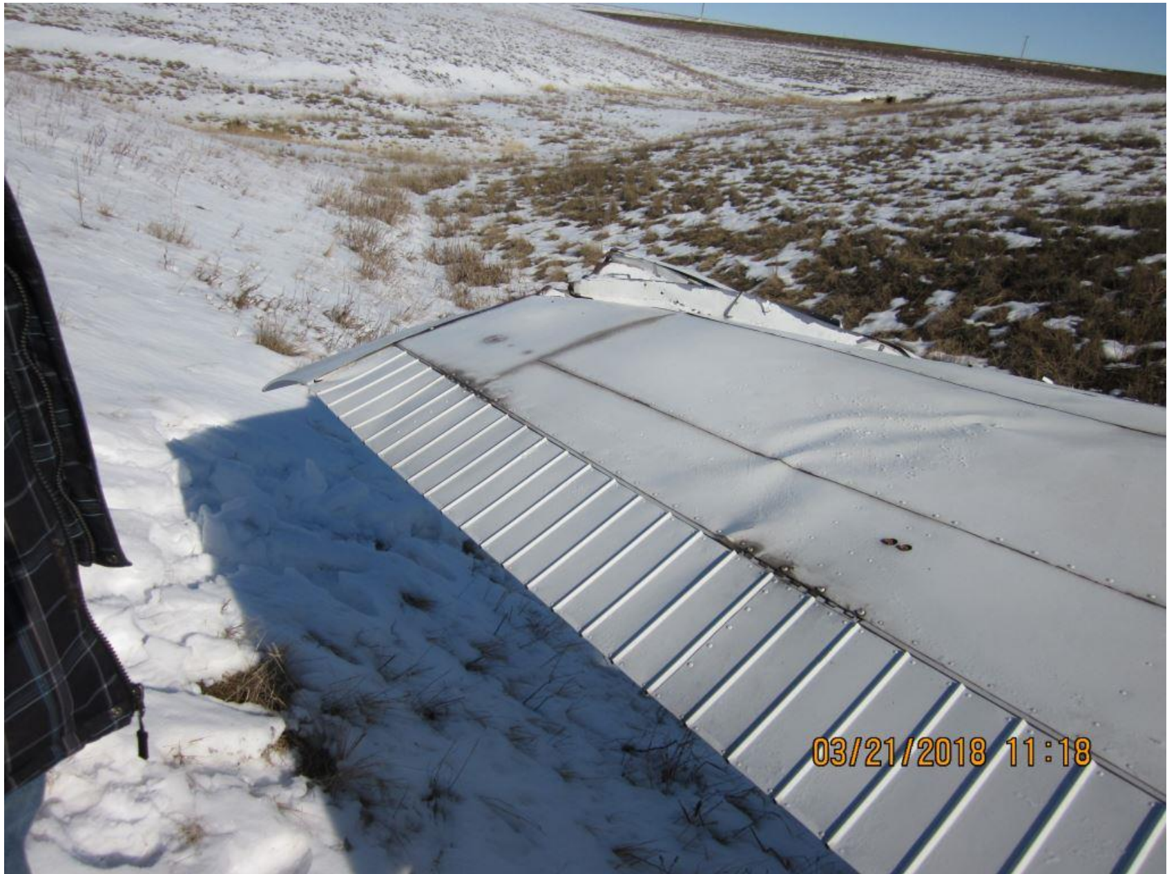
Photo 2 – View of damaged left wing and aileron (Photo courtesy of the FAA)
