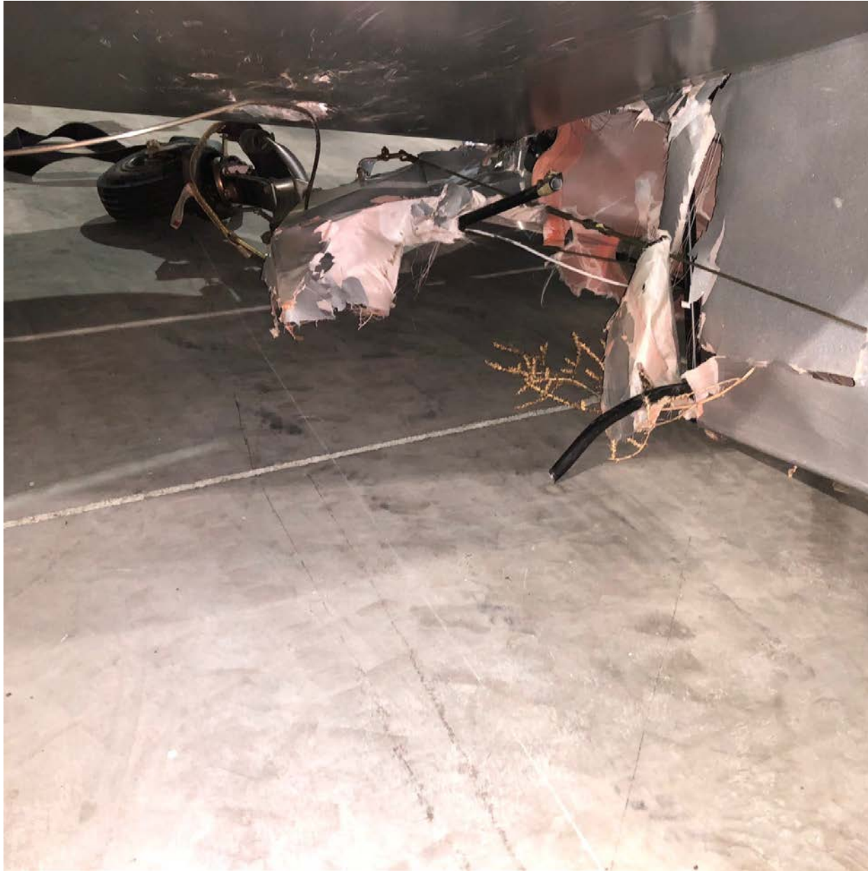
Photo 2 – View of damaged empennage (Photo courtesy of the pilot)
