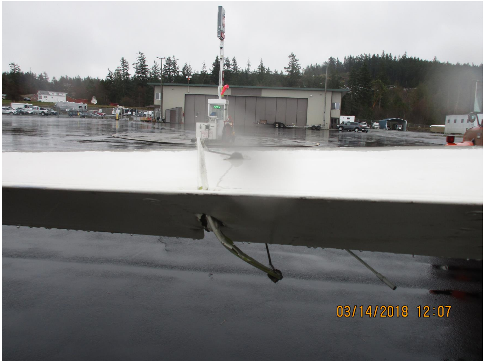
Photo 1 – View of damaged left aileron (Photo courtesy of the FAA)
