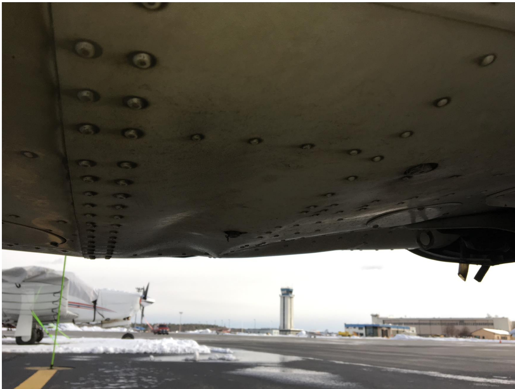
Photo 1 – View of damaged bottom fuselage (Photo courtesy of the FAA)
