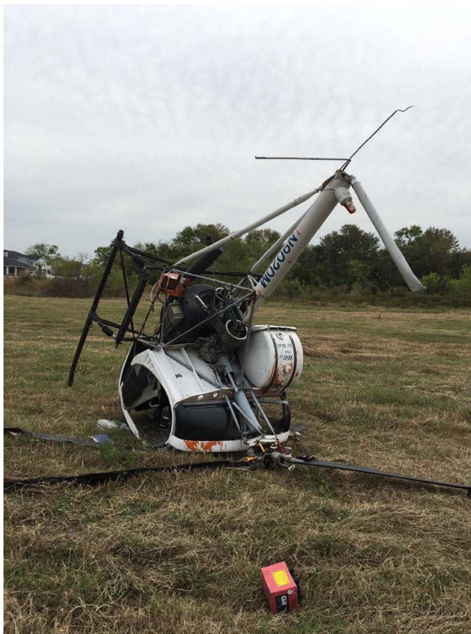
Photo 1 – View of damage to the main rotor and tail rotor drive system (Courtesy of FAA)
