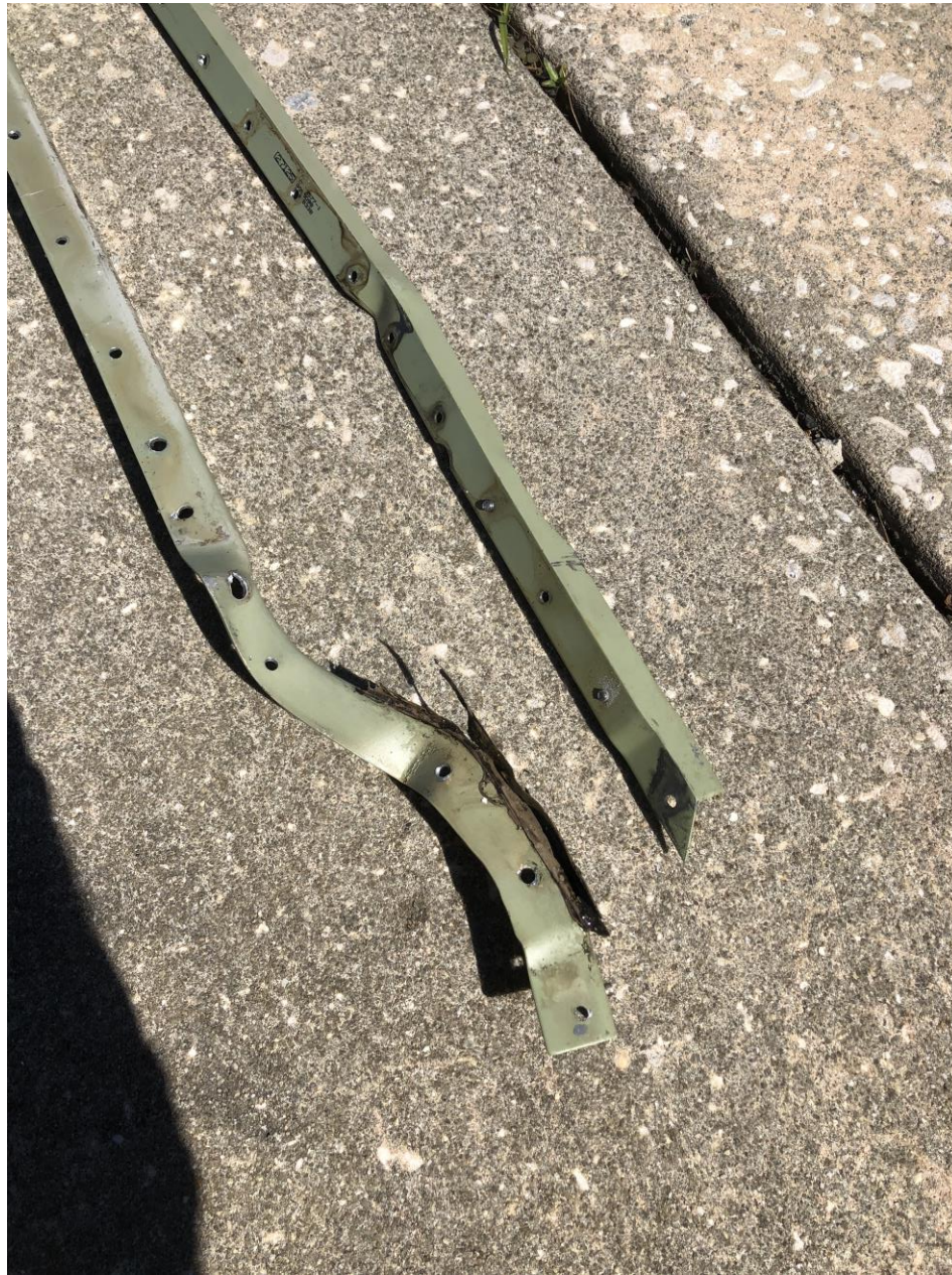
Photo 2 – View of removed floor stringers (Photo courtesy of the operator)
