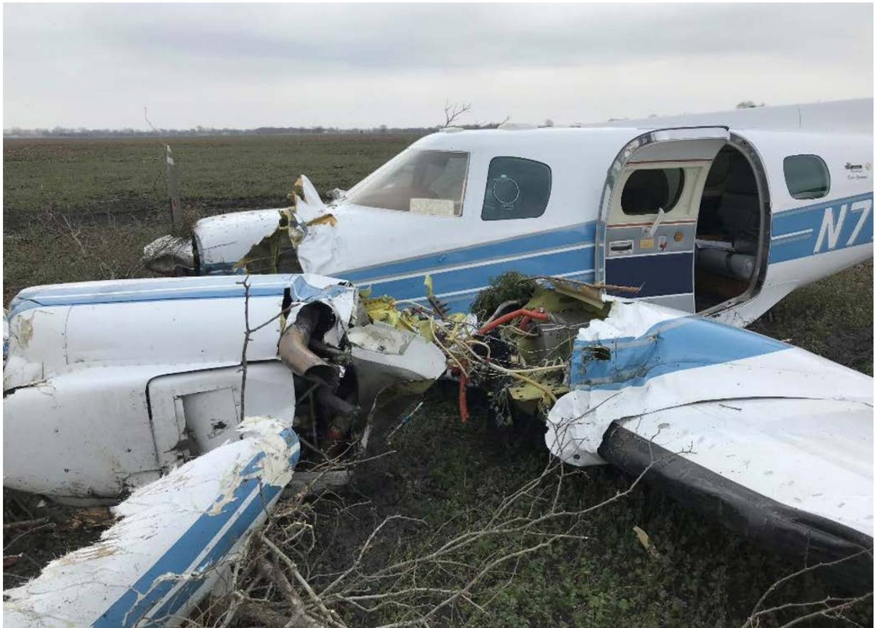
Photo 1 – View of damage to engine mounts (Courtesy of FAA)
