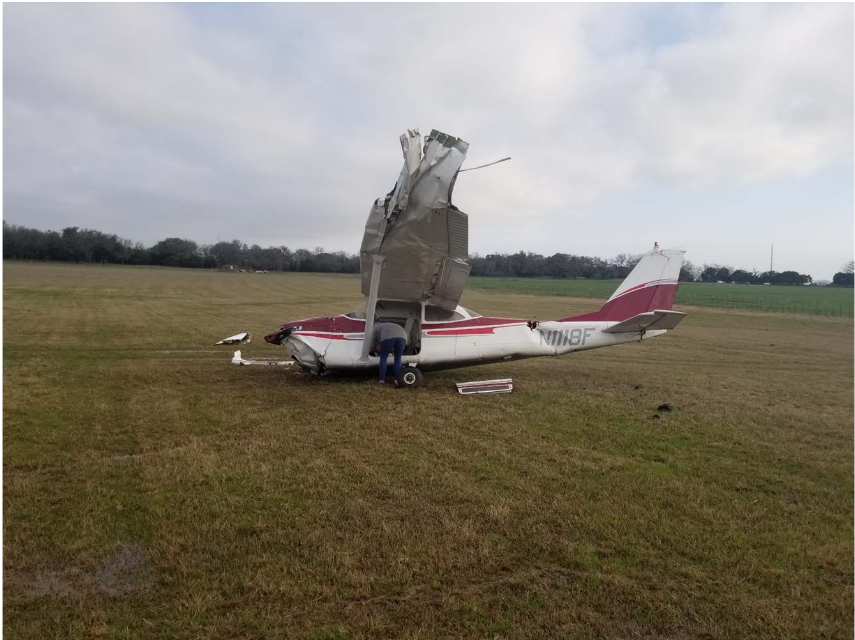
Photo 1 – View of damage to left wing and tail cone (Courtesy of FAA)
