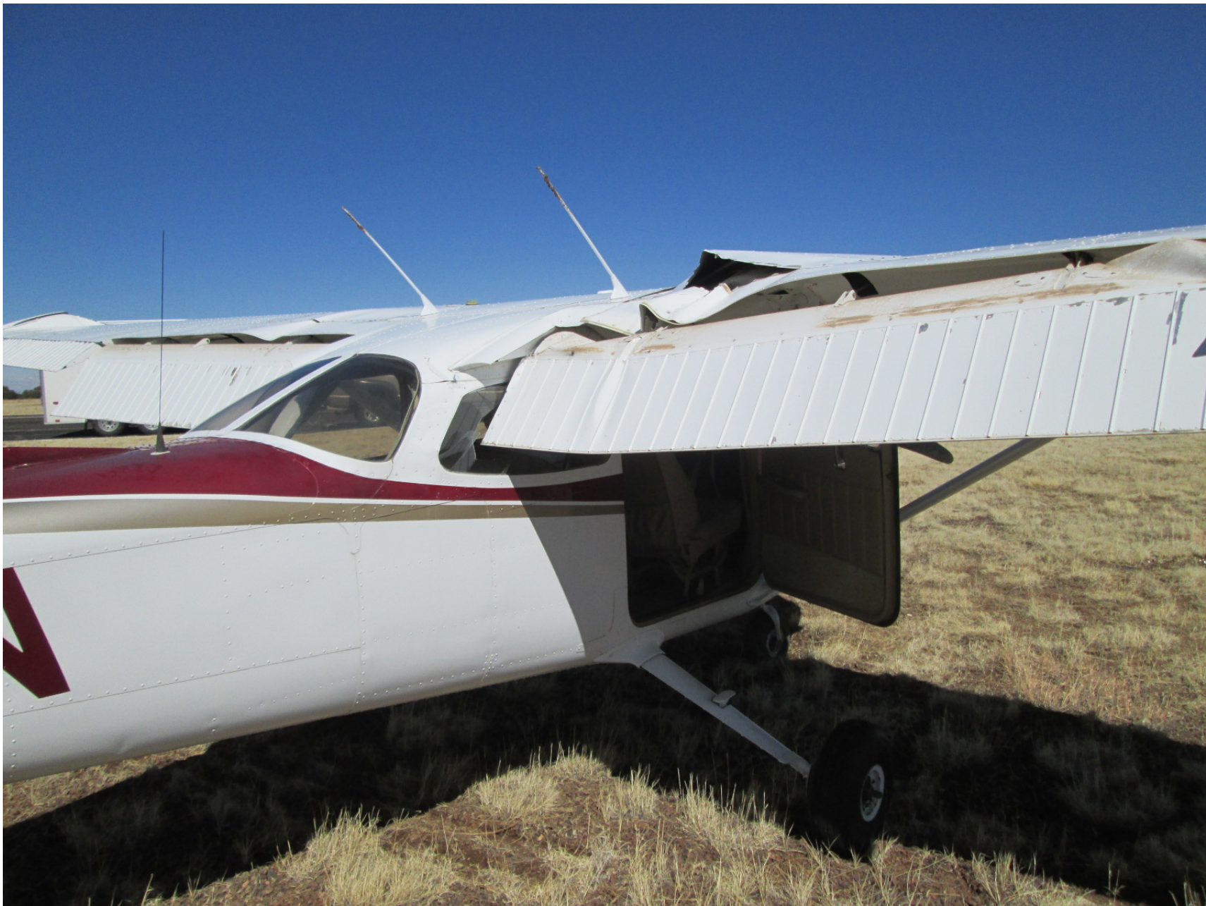
Photo 2 – View of damaged wings (Photo courtesy of the Airport Manager)
