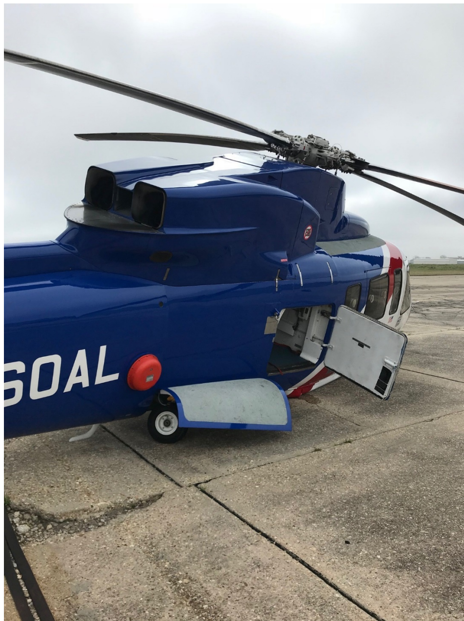
Photo 1 – View of collapsed right landing gear (Photo courtesy of the FAA)
