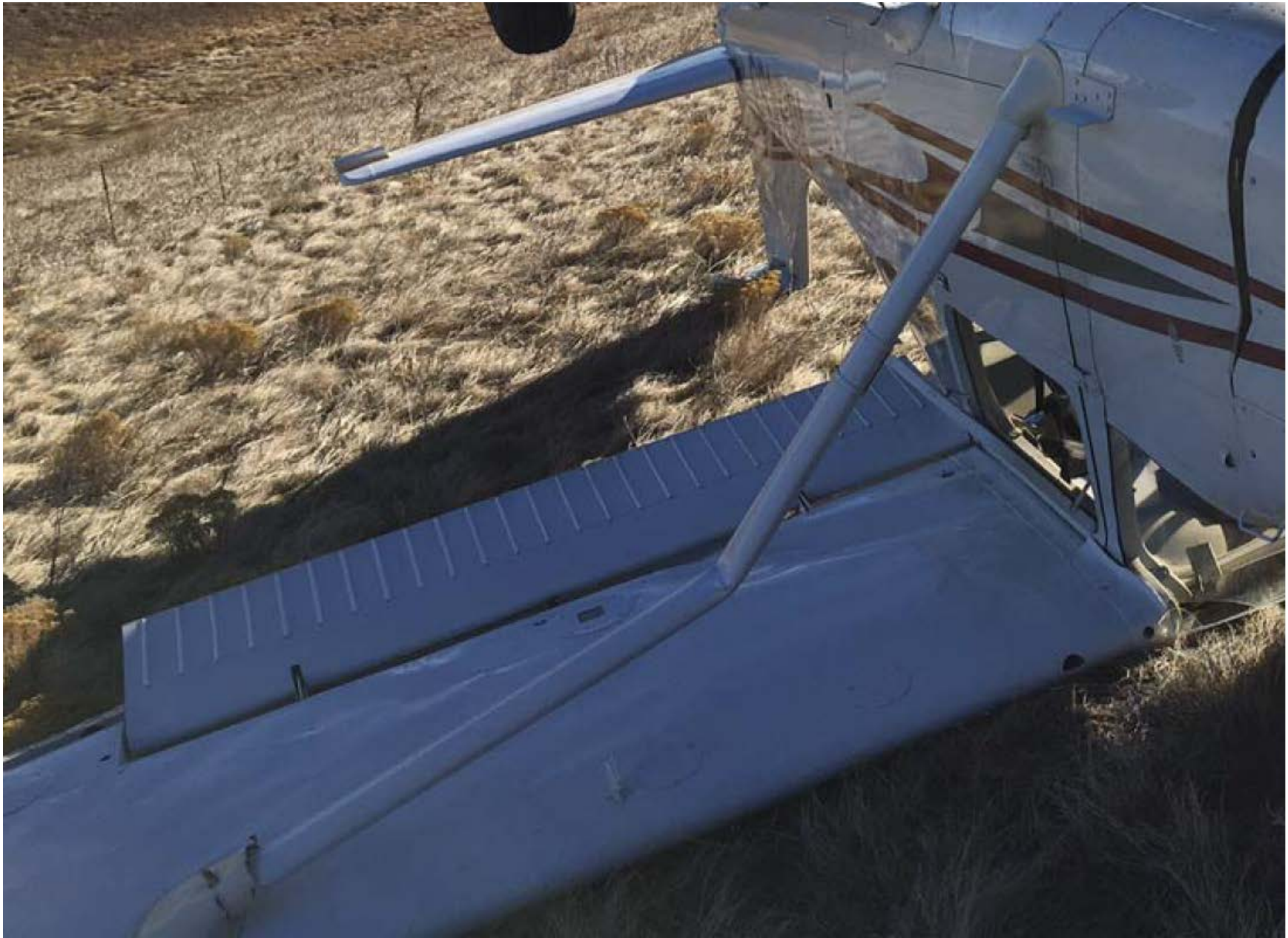
Photo 1 – View of damage to left wing lift strut and vertical stabilizer (Courtesy of FAA)
