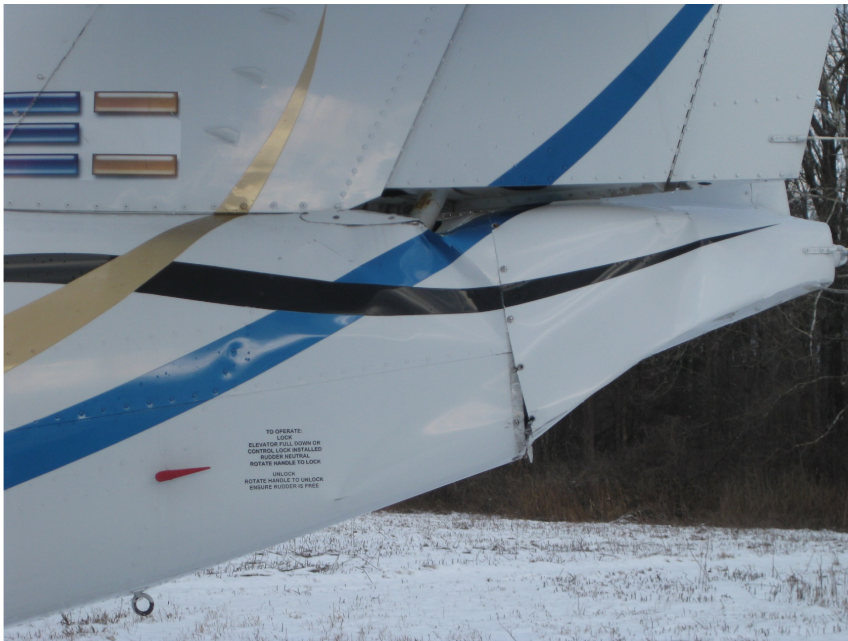
Photo 2 – View of damaged empennage (Photo courtesy unknown)
