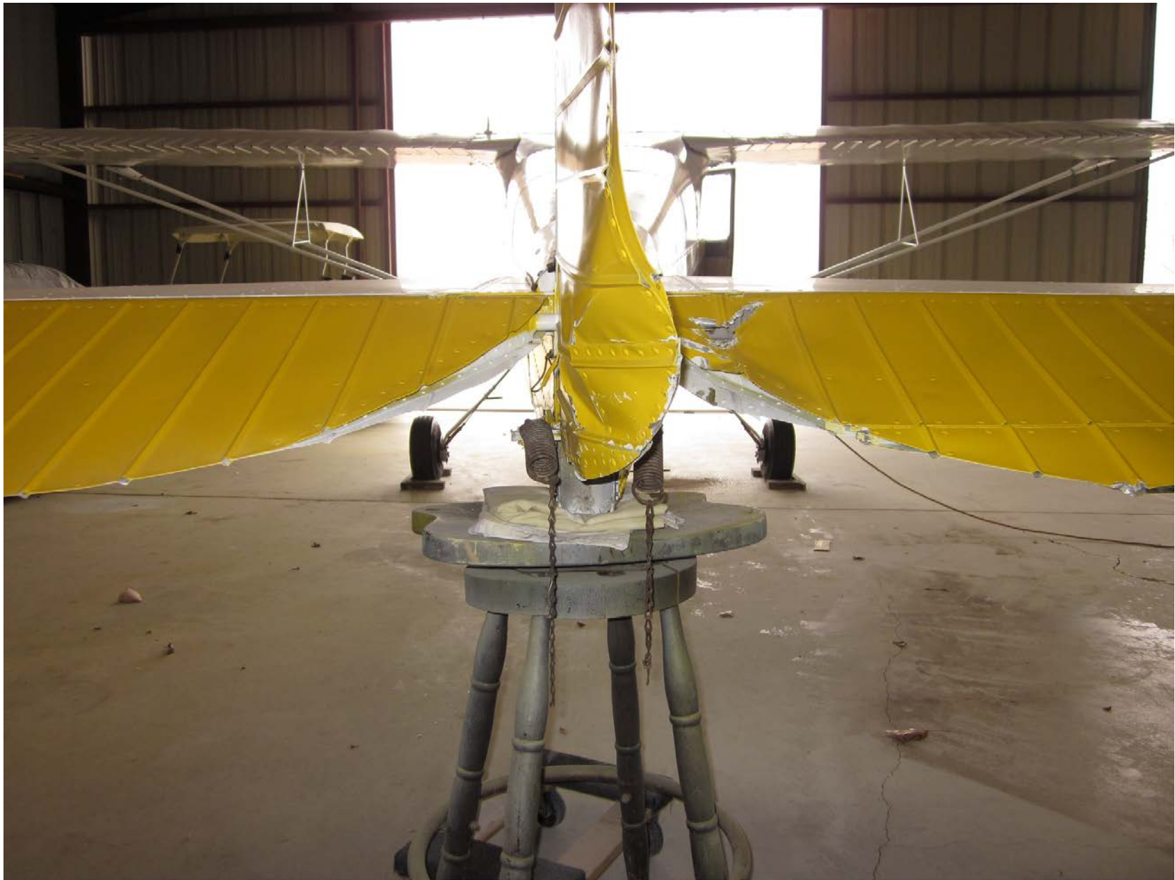
Photo 1 – View of damage to rudder and right elevator (Courtesy of FAA)
