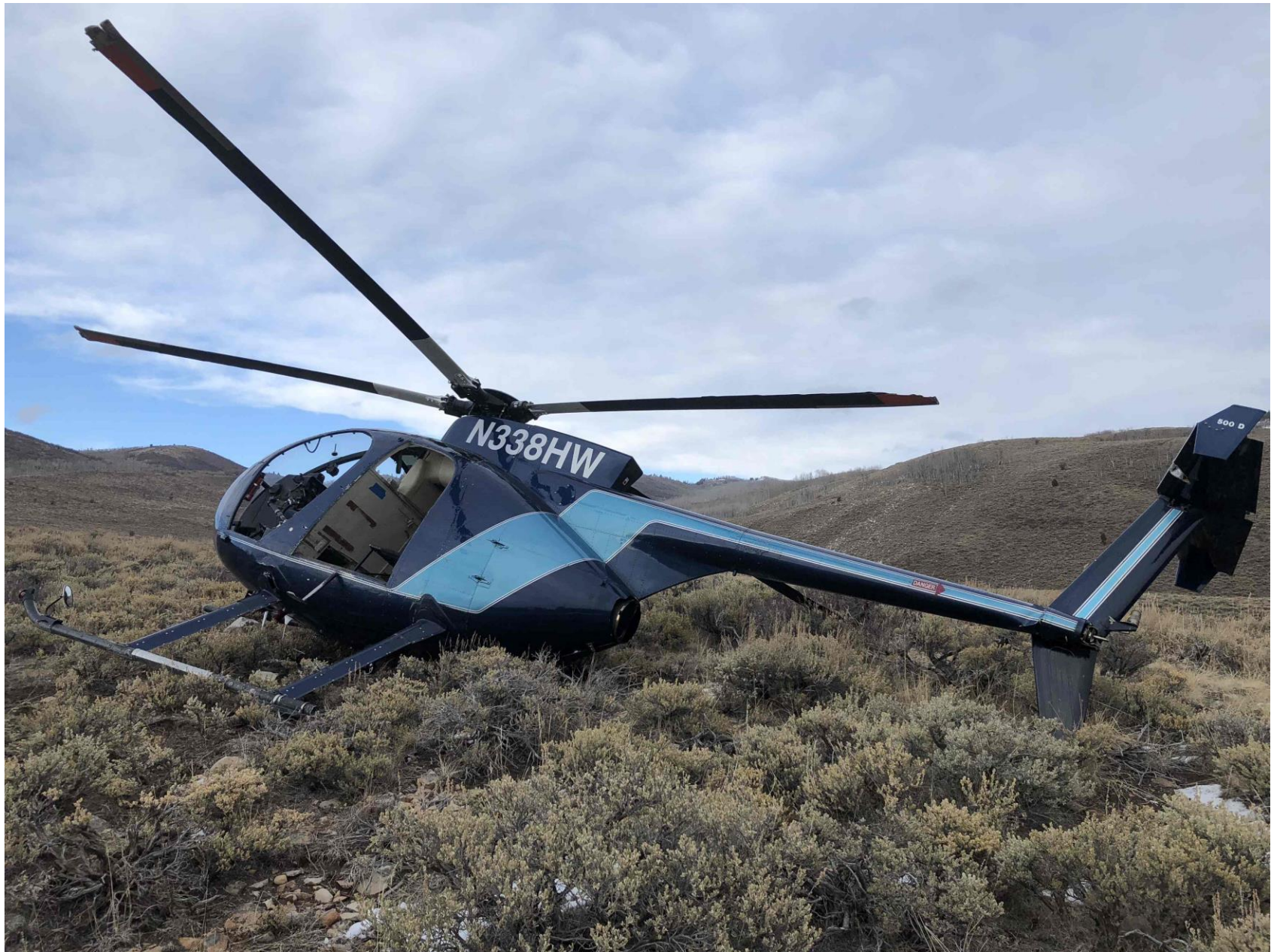
Photo 1 – View of accident helicopter and damaged tail rotor (Photo courtesy of the operator)
