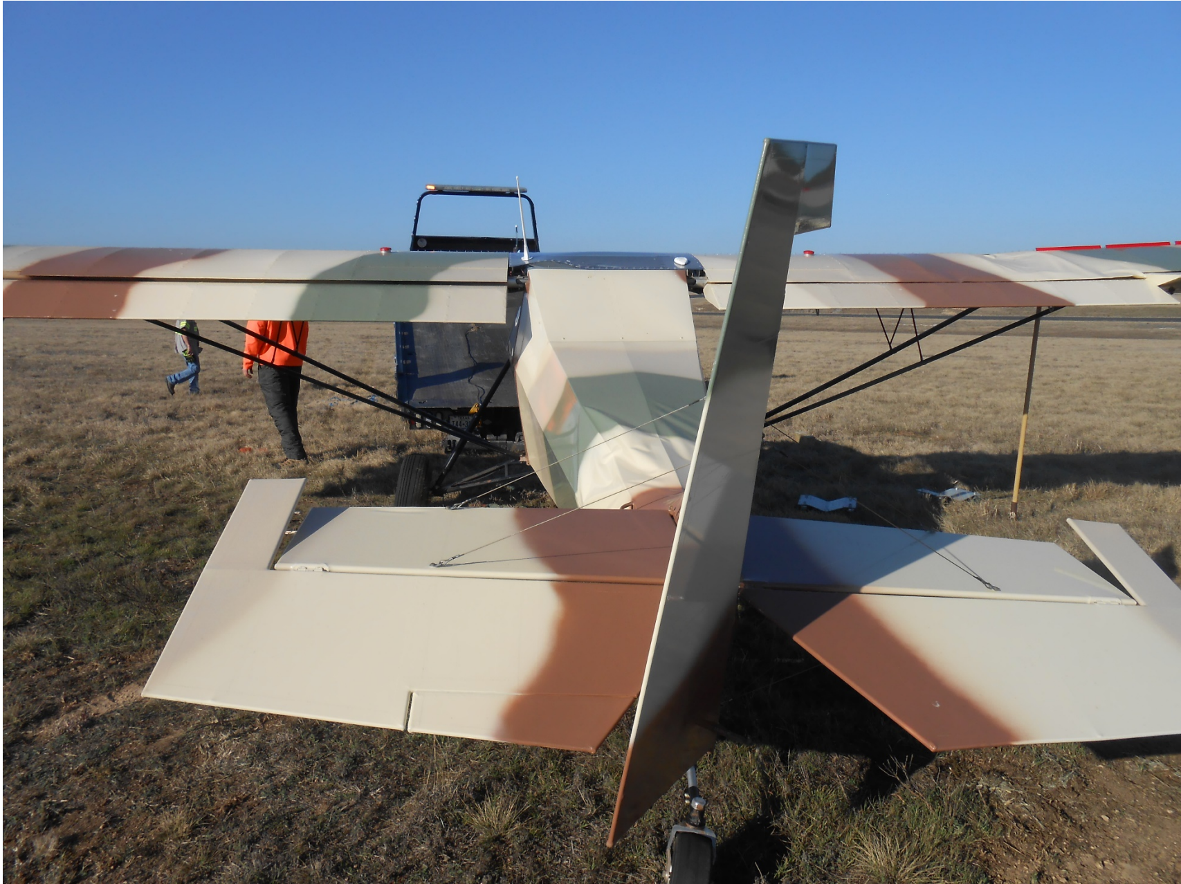
Photo 1 – View of damaged empennage from rear of airplane (Photo courtesy of the FAA)
