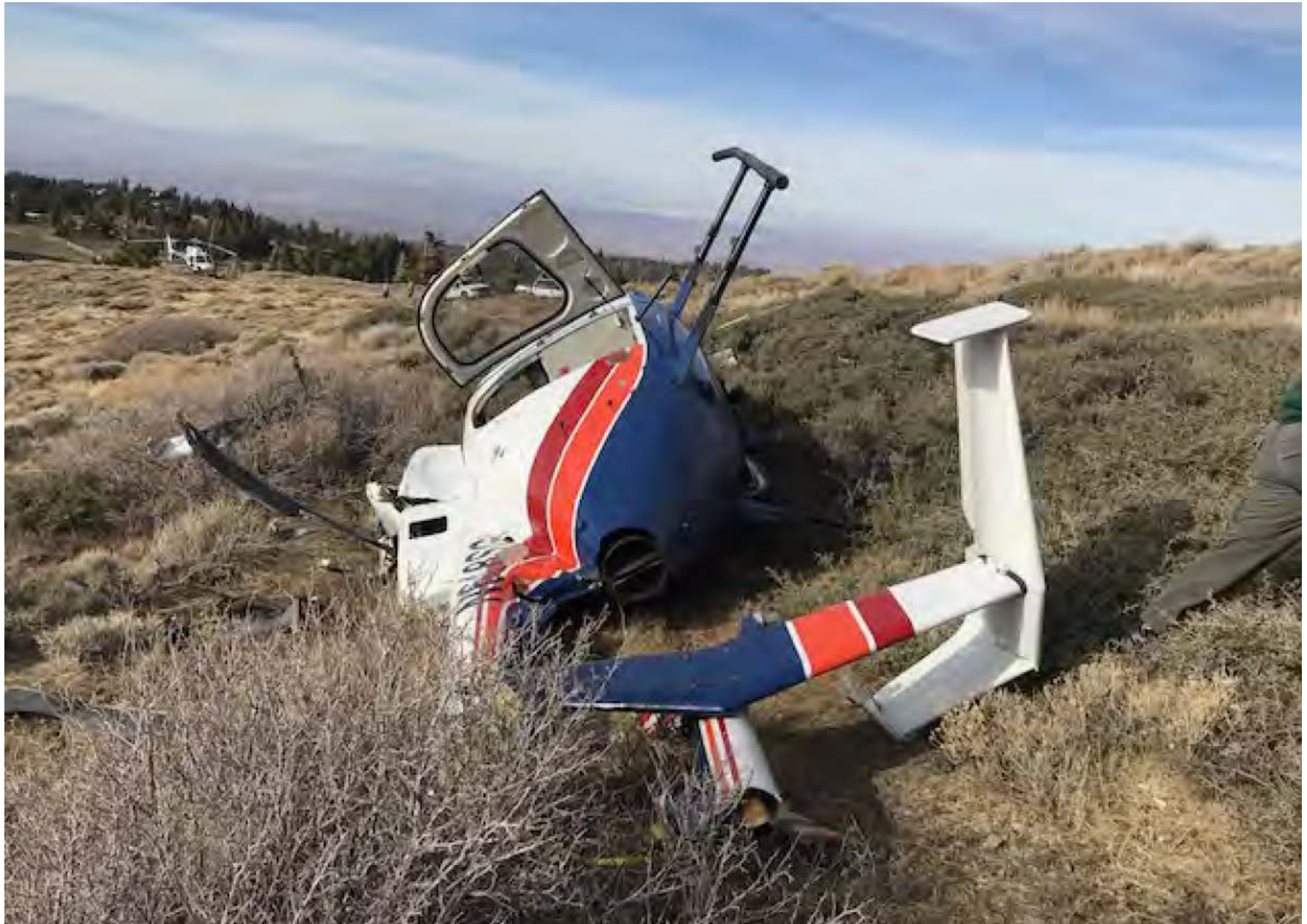
Photo 2 – View of damage to the tailboom (Courtesy of FAA)
