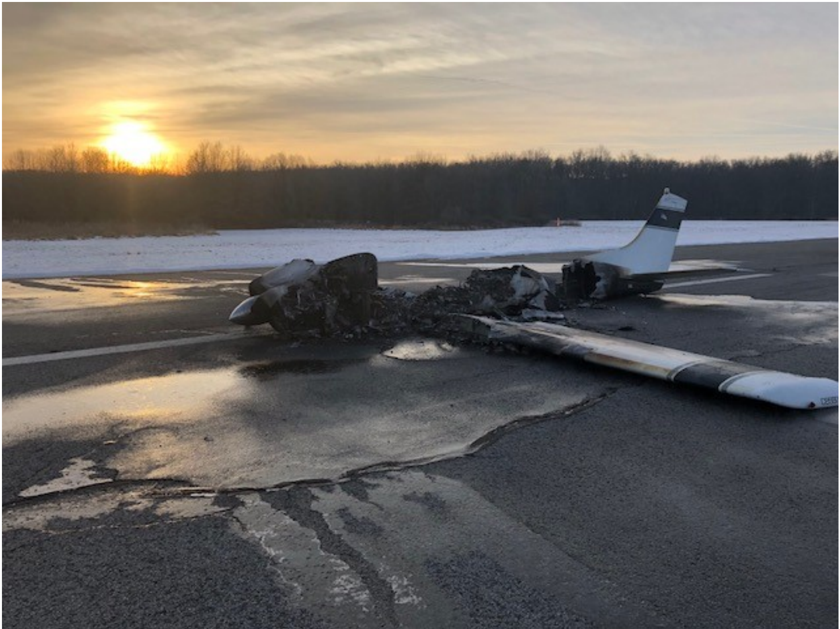
Photo 1 – View of destroyed airplane after postaccident fire (Photo courtesy unknown)
