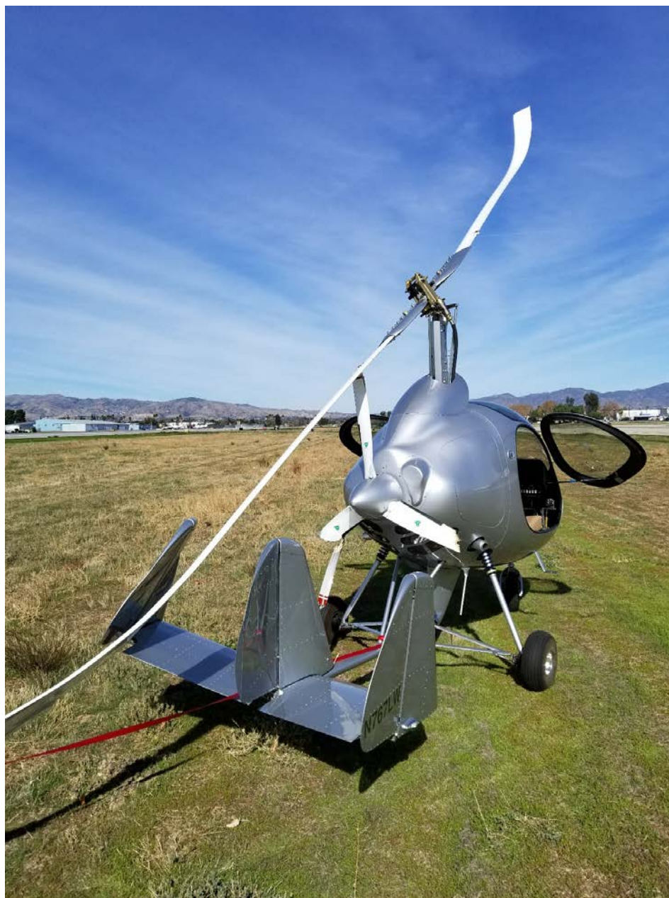
Photo 1 – View of damage to the left vertical stabilizer (Courtesy of FAA)
