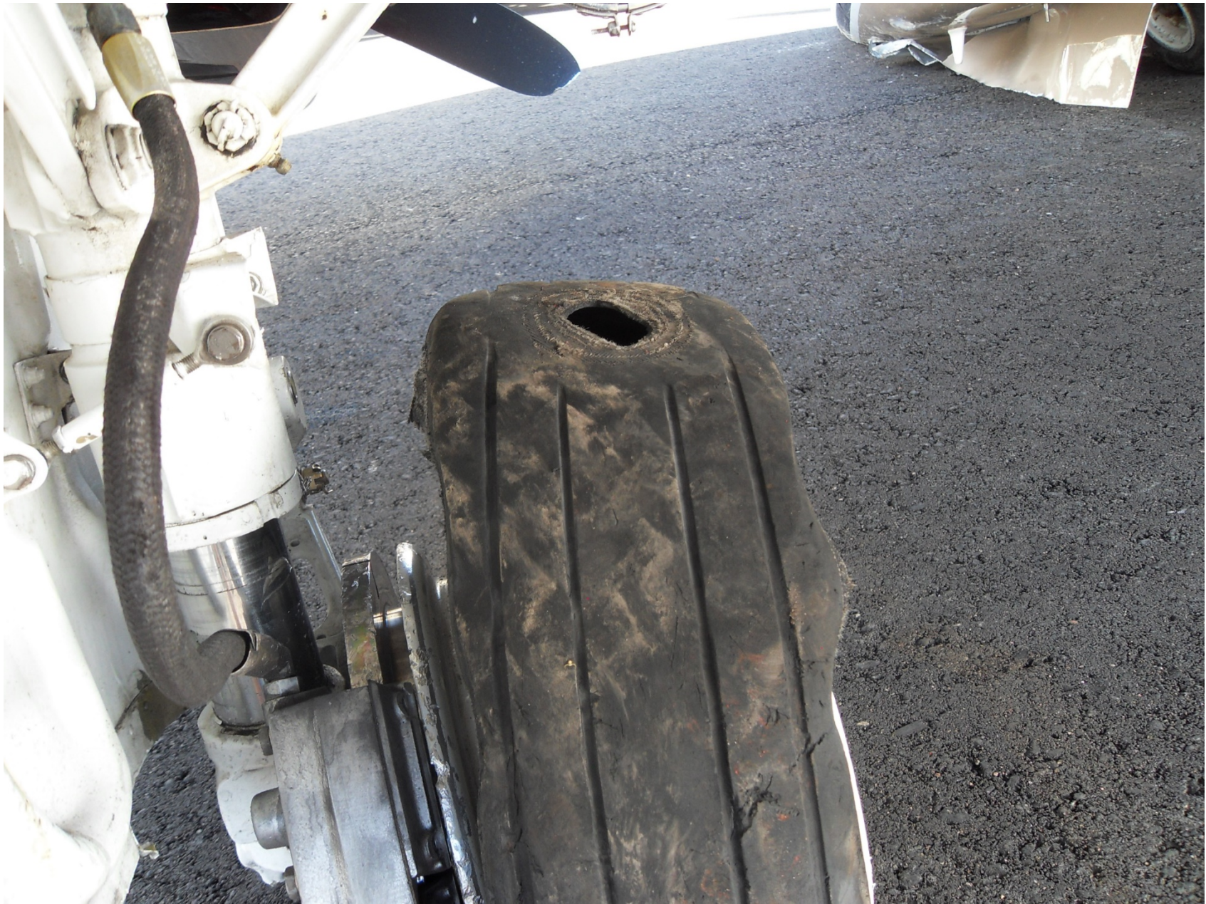
Photo 2 – View of hole in left main landing gear tire (Photo courtesy of the FAA)
