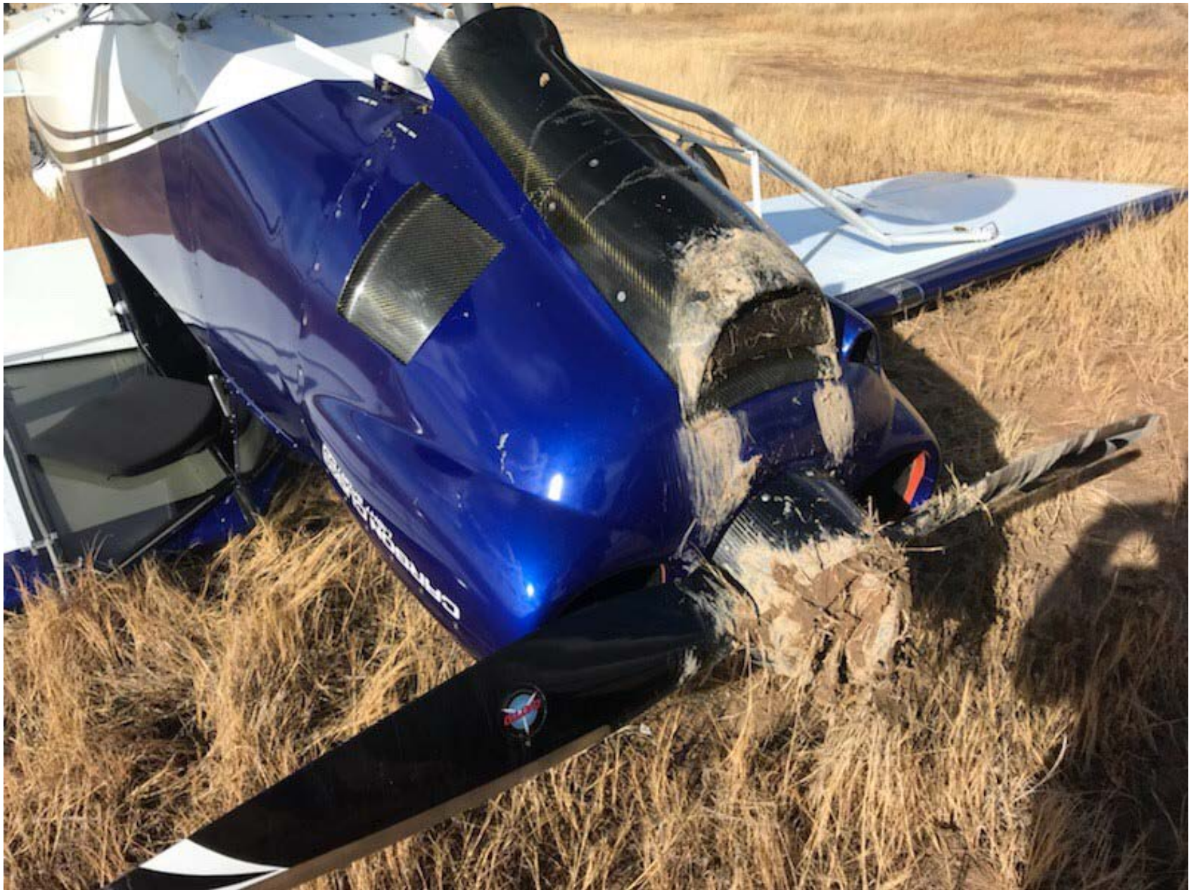
Photo 2 – View of damage to right wing lift strut (Courtesy of FAA)
