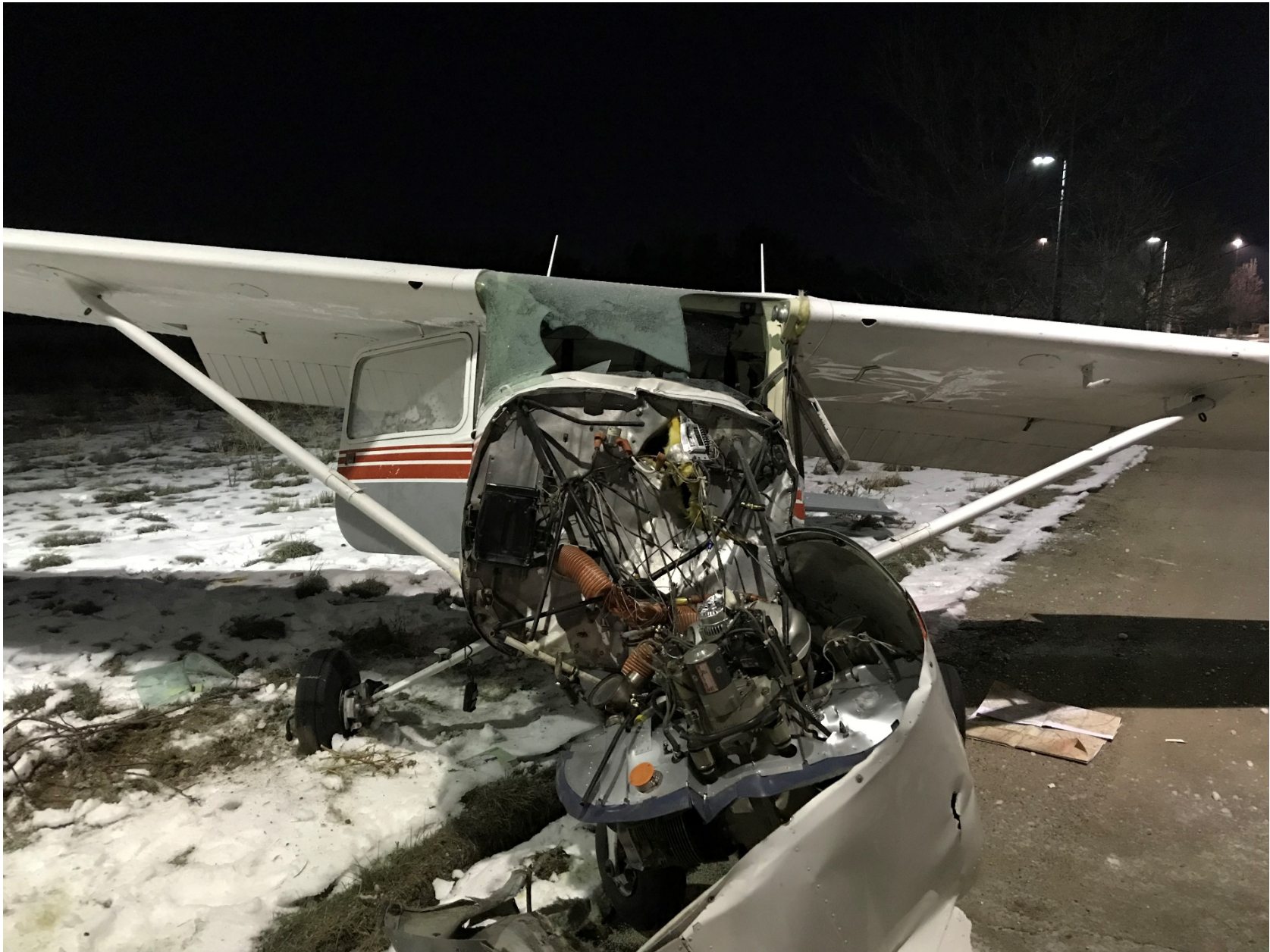
Photo 2 – View of damaged windscreen and engine compartment (Photo courtesy of local law enforcement)
