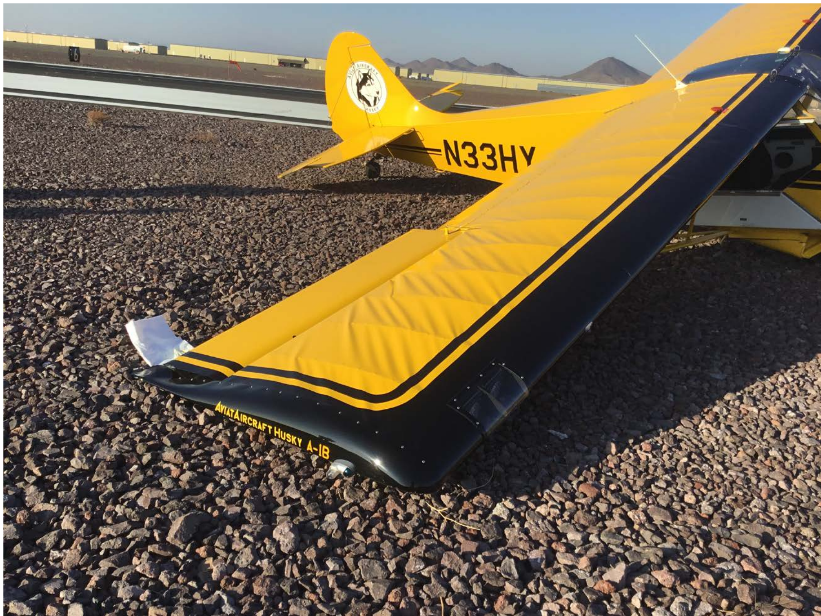
Photo 1 – View of damage to right wing and collapsed landing gear assembly (Courtesy of FAA)
