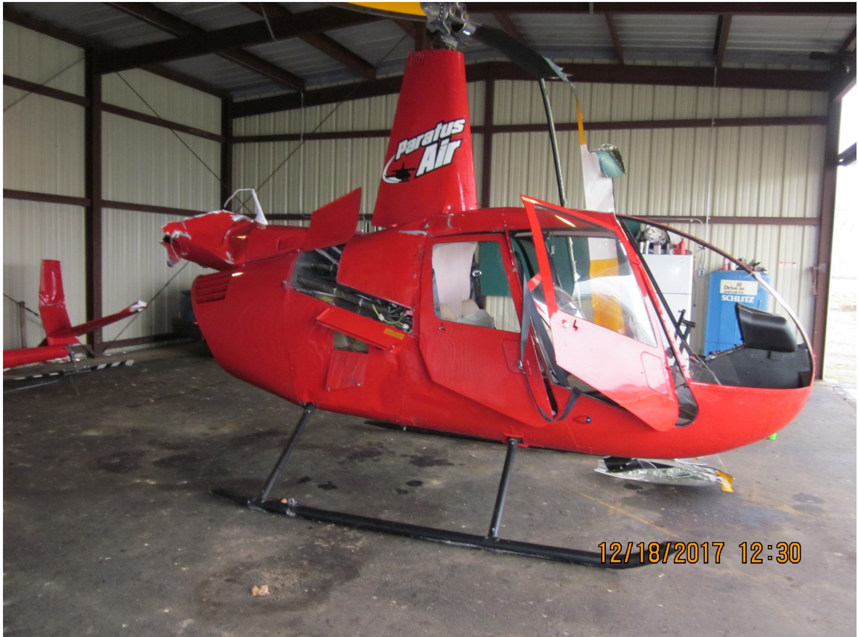
Photo 1 – View of damaged tail boom and main rotor blade (Photo courtesy of the FAA)
