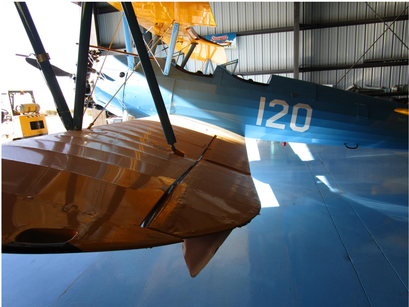
Photo 1 – View of damaged aileron (Photo courtesy of the FAA)
