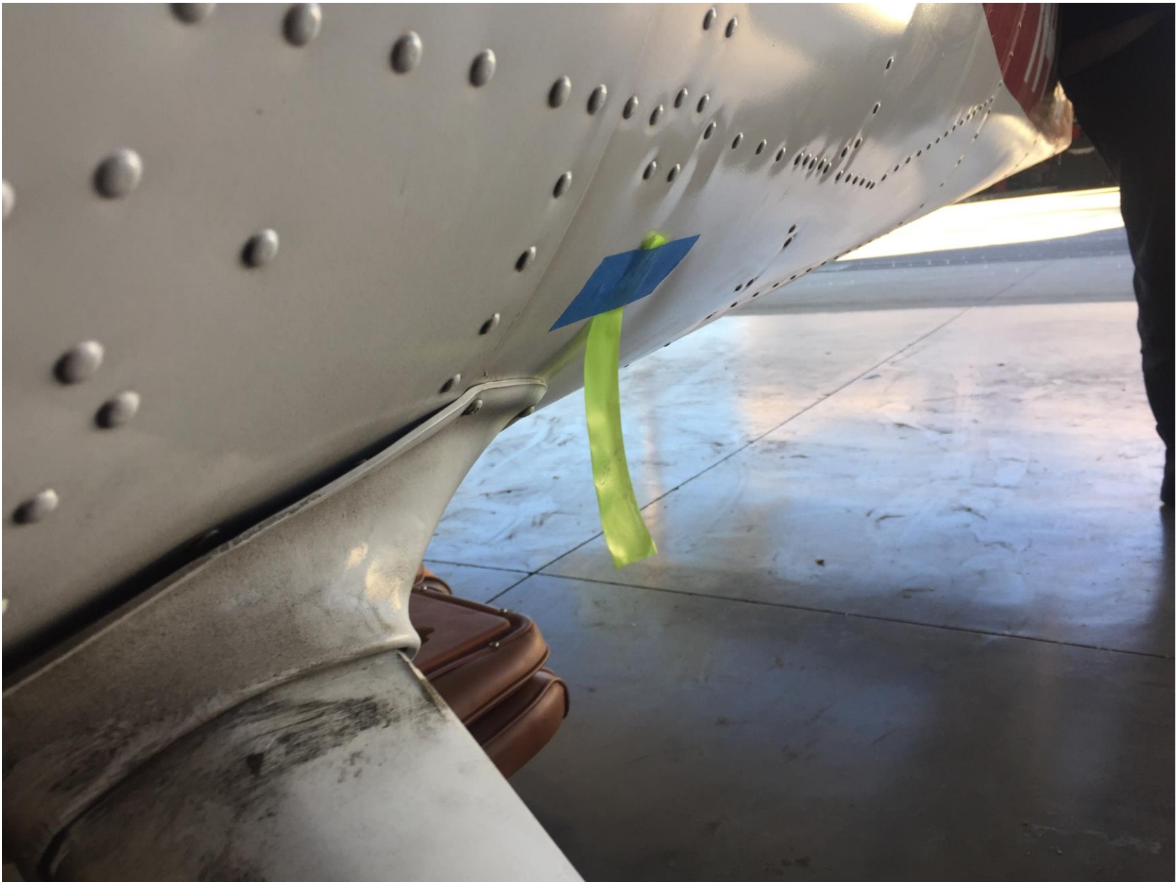
Photo 2 – View of wrinkled fuselage aft of the main landing gear (Photo courtesy of the FAA)
