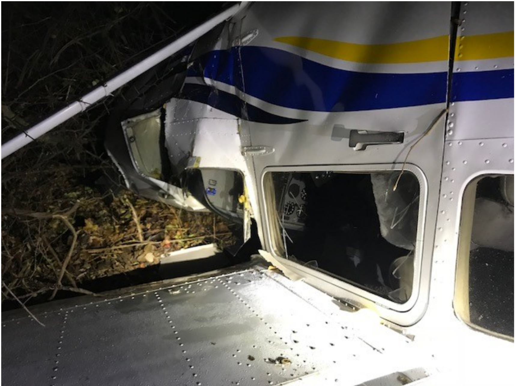
Photo 2 – View of damaged fuselage of inverted airplane (Photo courtesy of the FAA)
