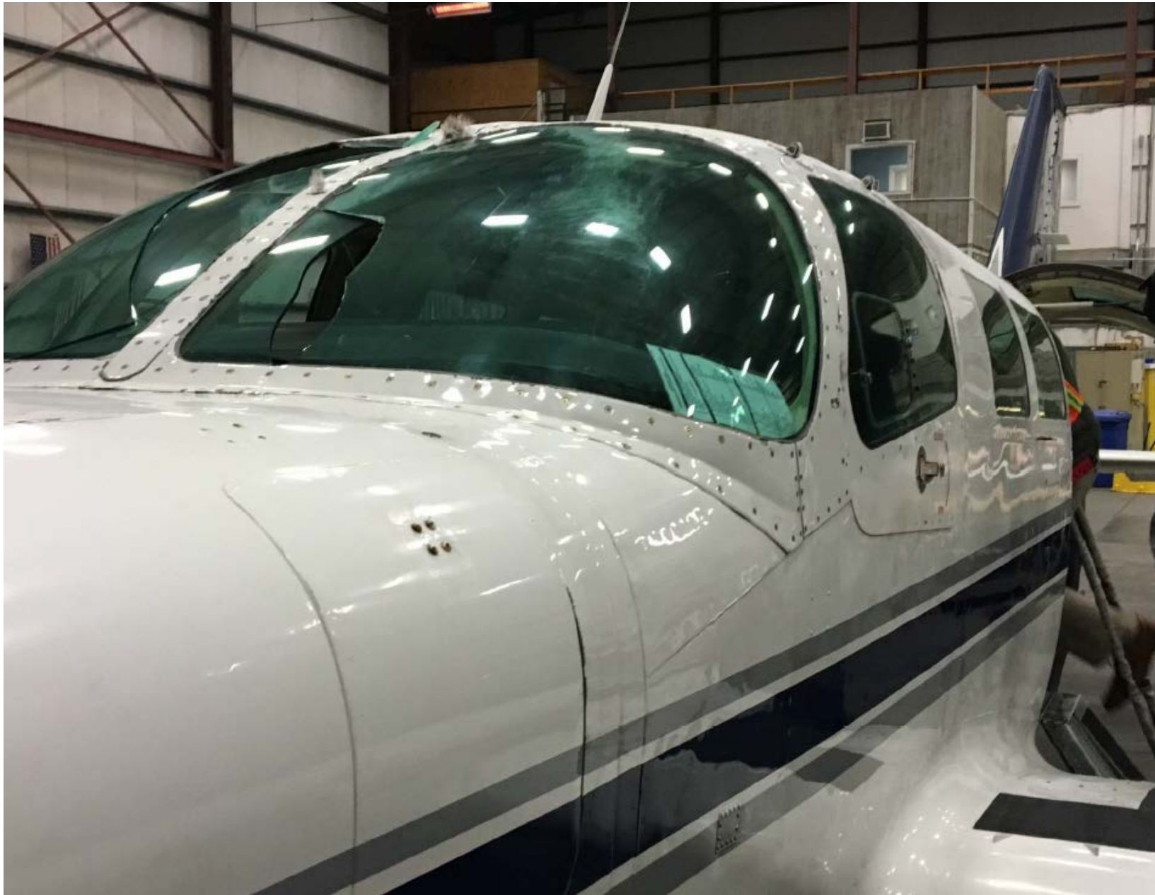
Photo 1 – View of damage to the windscreen (Courtesy of FAA)
