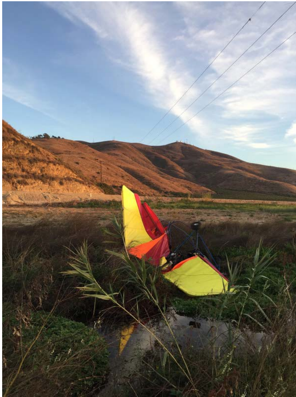
Photo 1 – View of damaged airplane under power wires (photo courtesy of the FAA)
