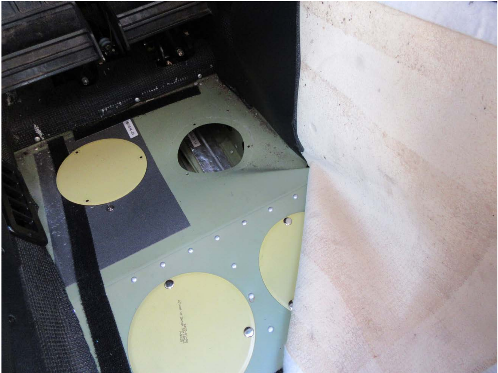
Photo 2 – View of damaged floorboard (photo courtesy of the FAA)
