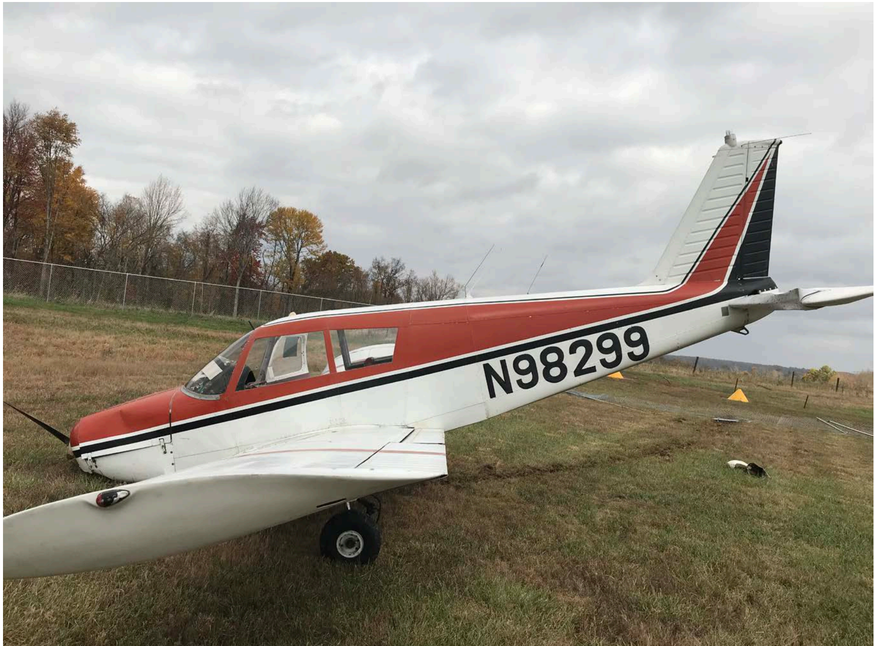
Photo 1 – View of airplane after striking airport fence (photo courtesy of the FAA)
