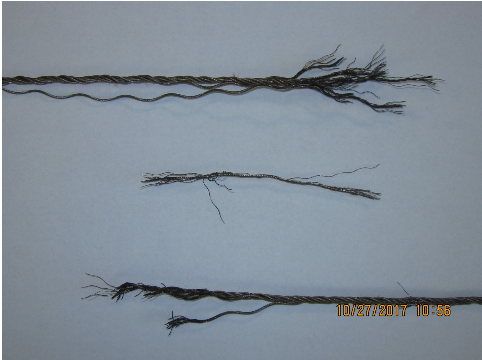
Photo 3 – View of three sections of separated rudder (photo courtesy of the FAA)
